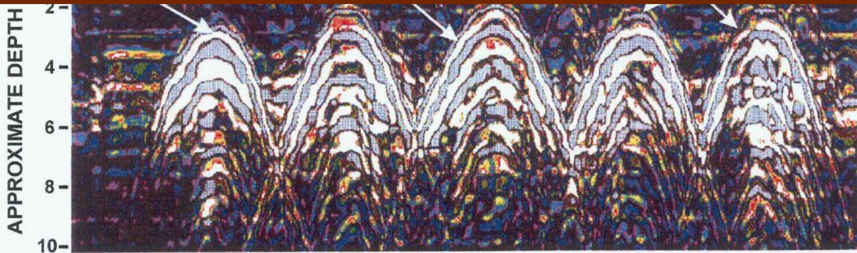
GPR Survey to Locate Underground Storage Tanks
