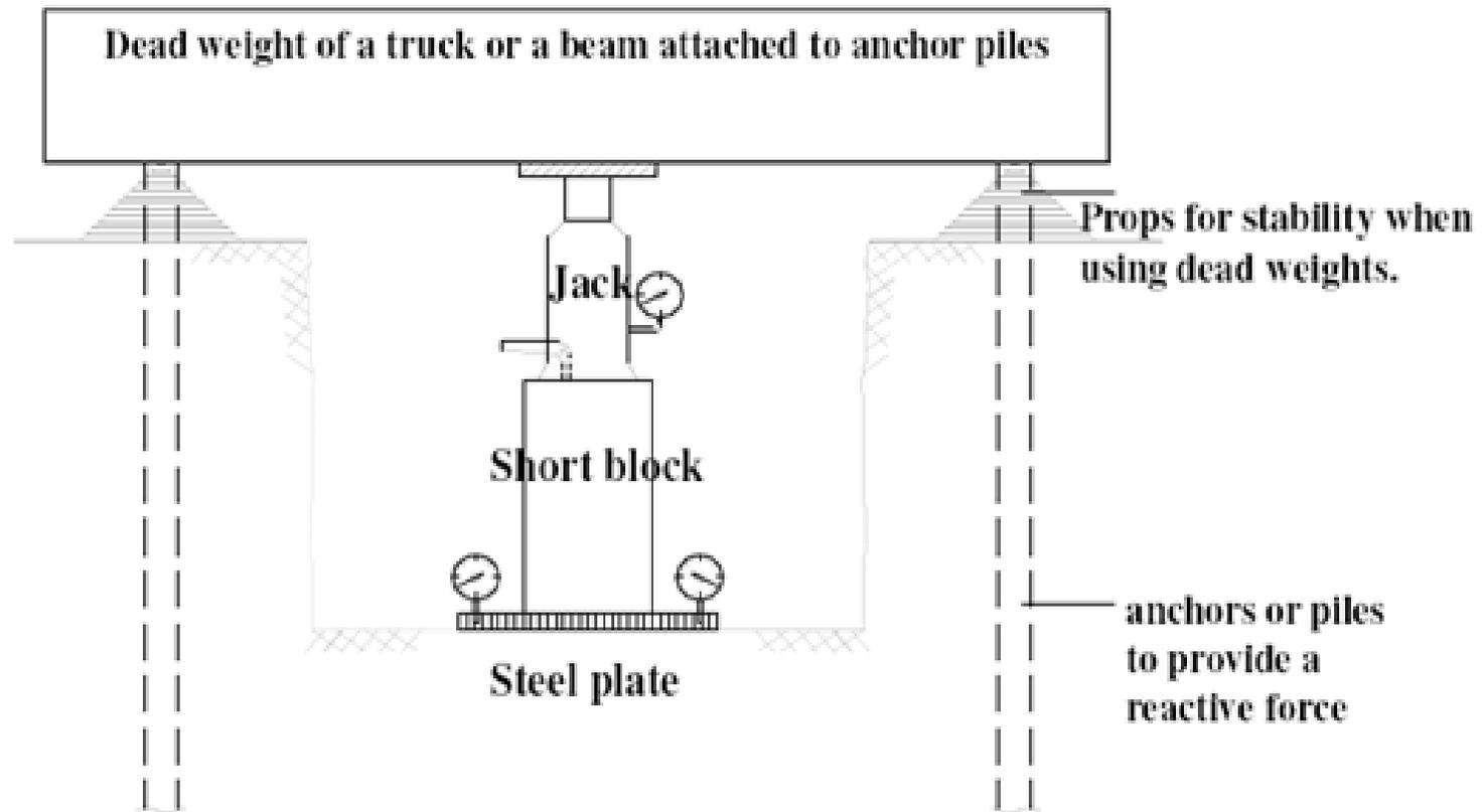
Several dial gauges attached to an independent suspension system to record plate settlements with each increment of the jack load.
