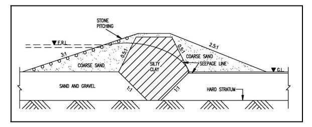
Fig. 23: Typical Earth Dam Section with Coarse Sand
