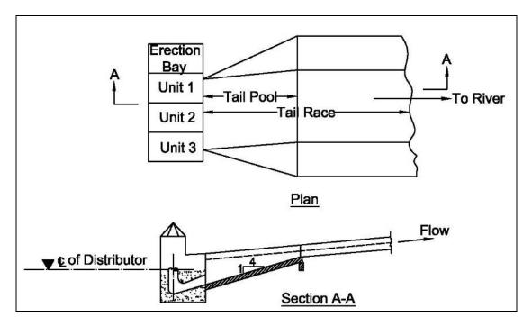
Fig. 68: Typical tailrace for high Discharge Installation
