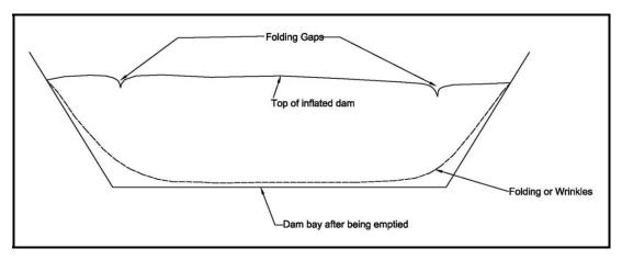
Fig. 15: Folding gaps or Wrinkles of Conventional Rubber Dam
