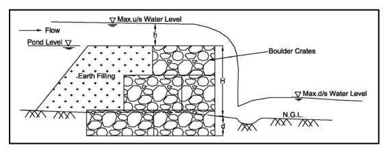
Fig. 3 (a): Typical Section of Gabion Weir
