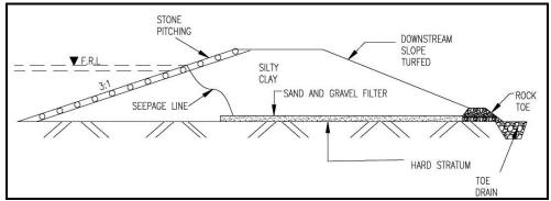
Fig. 19: Typical Section with Silty Clay
