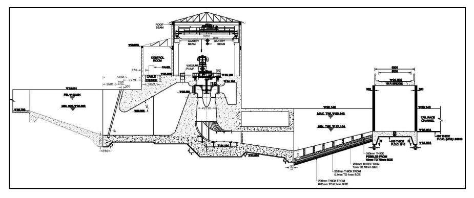
Fig. 67: Typical Transverse Section of Power House with Syphon Kaplan Turbine
