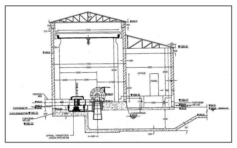
Fig. 63: Typical Transverse Section of Power House with Horizontal Francis Turbine
