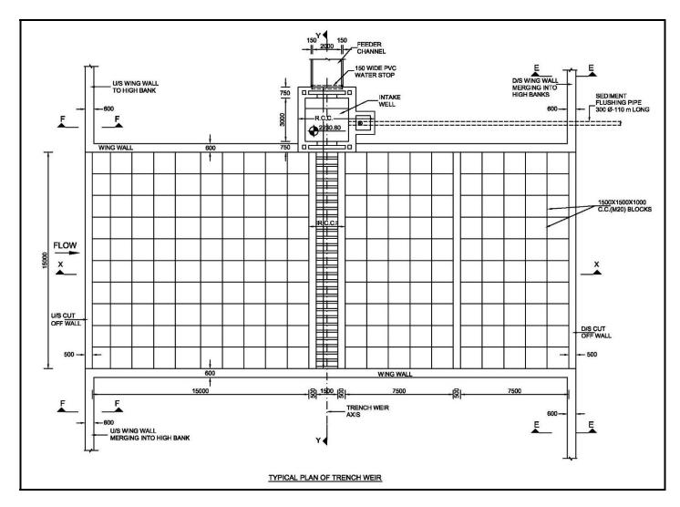
Fig. 5 (a): Typical Details of Trench Weir (Plan)
