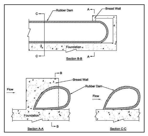
Fig.16: Breast Wall Arrangement
