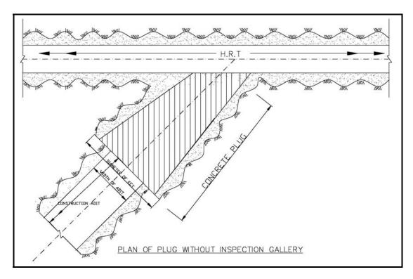
Fig. 48: Details of Plug without Inspection Gallery
