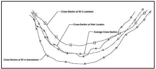
Fig. 1: Determination of Average River Section
