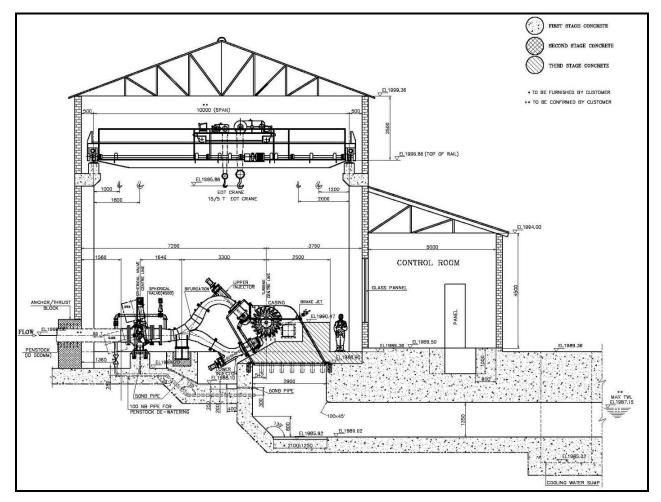
Fig. 64: Typical Transverse Section of Power House with Horizontal Pelton Turbine
