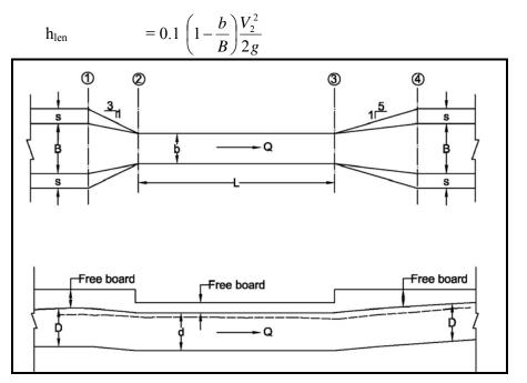
Fig. 51: Geometric Layout of Flumed Aqueduct
