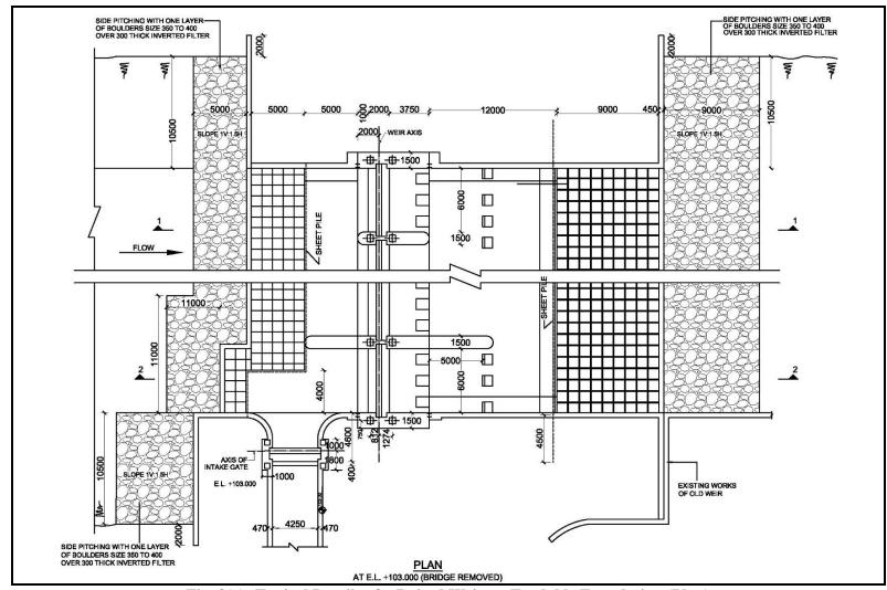
Fig. 8(a): Typical Details of a Raised Weir on Erodable Foundation (Plan)
