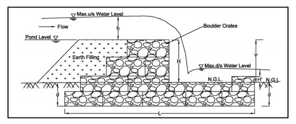
Fig. 3 (b): Typical Section of Gabion Weir with Downstream Protection Works
