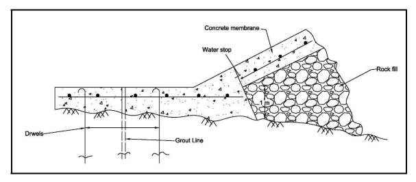
Fig. 21: Typical Details of a Cut off / Plinth
