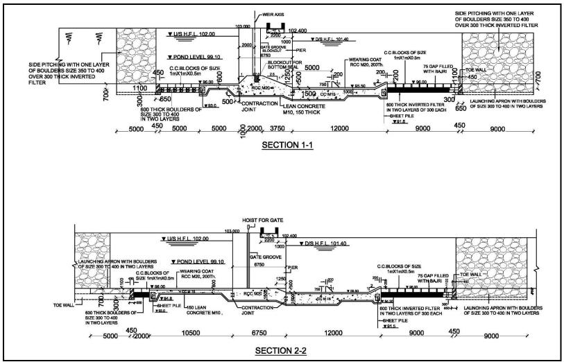
Fig. 8(b): Typical Details of a Raised Weir on Erodable Foundation (Section)
