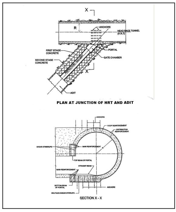
Fig. 47: Details of Plug with Inspection Gallery
