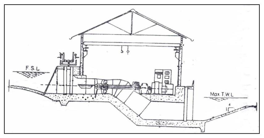
Fig. 65: Typical Transverse Section of Power House with Tubular Turbine
