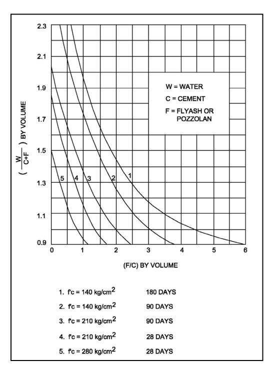
Fig. 11: Proportioning Curves for Equal Strength Concrete (R-37)
