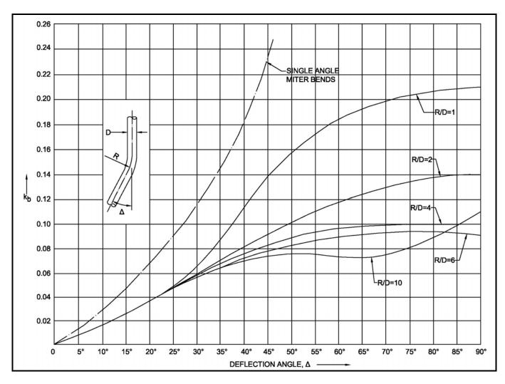
Fig. 58: Loss Coefficients for Pipe Bends of Smooth Interior (Source IS: 2951 (Part II) – 1965 (Reaffirmed 2003))
