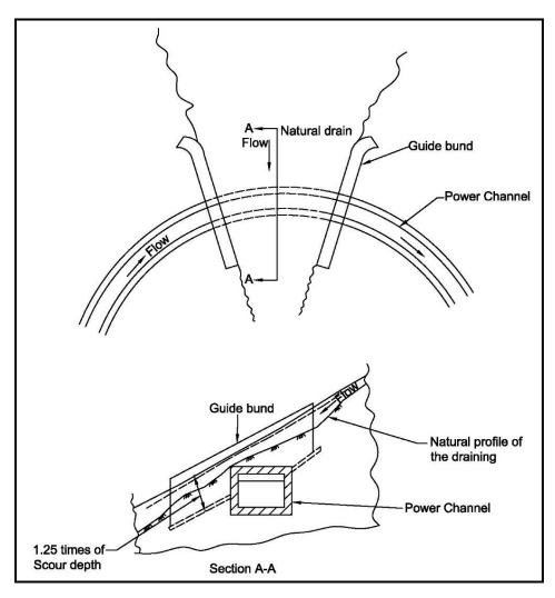
Fig. 49: Typical Arrangement of drain crossing above power channel
