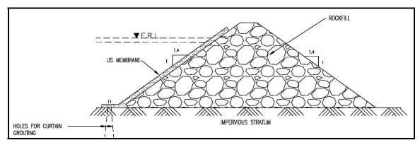
Fig. 20: Typical Section through Rockfill Dam
