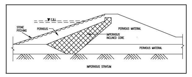
Fig. 24: Typical Earth Dam Section with Pervious Foundation upto Small Depth
