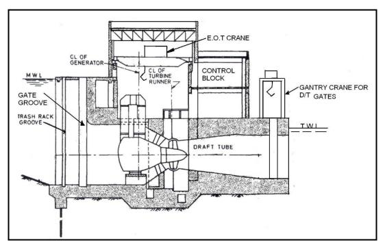
Fig. 31: Canal / River Power House Intakes (Bulb Turbines)
