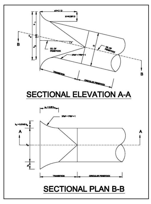
Fig. 35: Typical shape of intake opening
