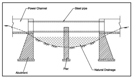
Fig. 53: Typical Section of Pipe Aqueduct
