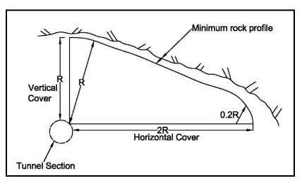
Fig. 46: Minimum Rock Cover in Power Tunnels
