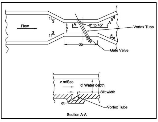
Fig. 55: General Arrangement of Vortex Tube
