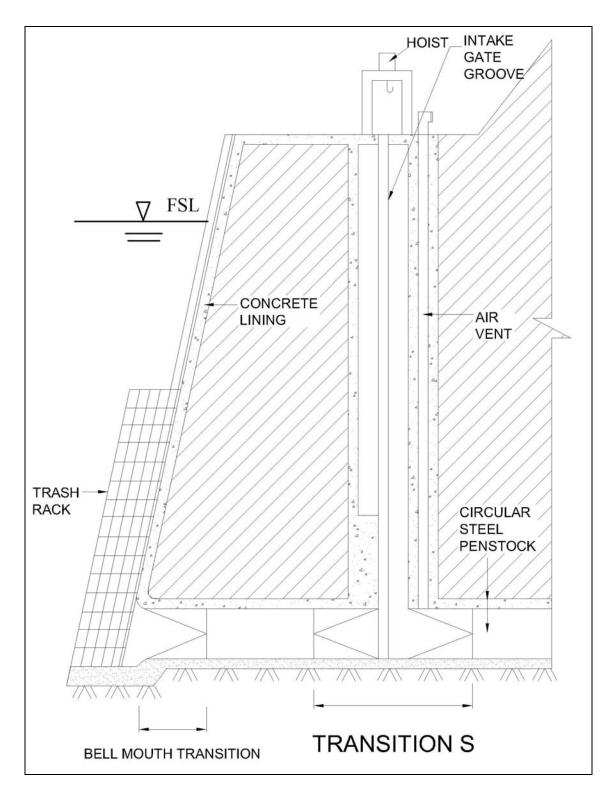
Fig. 34: Intake in Reservoir Independent of Dams
