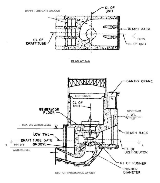
Fig. 30: Canal / River Power House Intakes (Kaplan Turbines)
