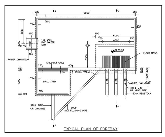
Fig. 57 (a): Typical Details of Forebay (Plan)
