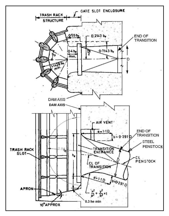
Fig. 33: Semi Circular Type Intake Structure
