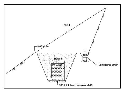
Fig. 43: Typical Section of Cut & Cover RCC Channel
