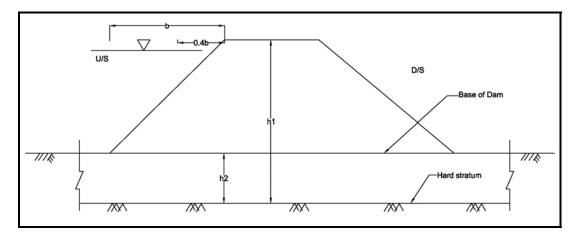
Fig. 28: Upstream and Downstream Slopes of the Dam
