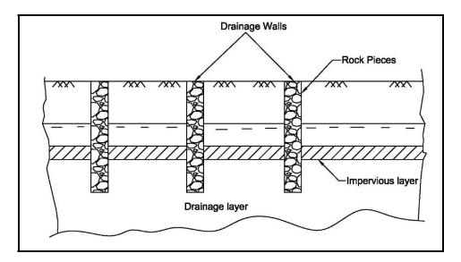
Fig. 39: Arrangement of Lowering Water Table
