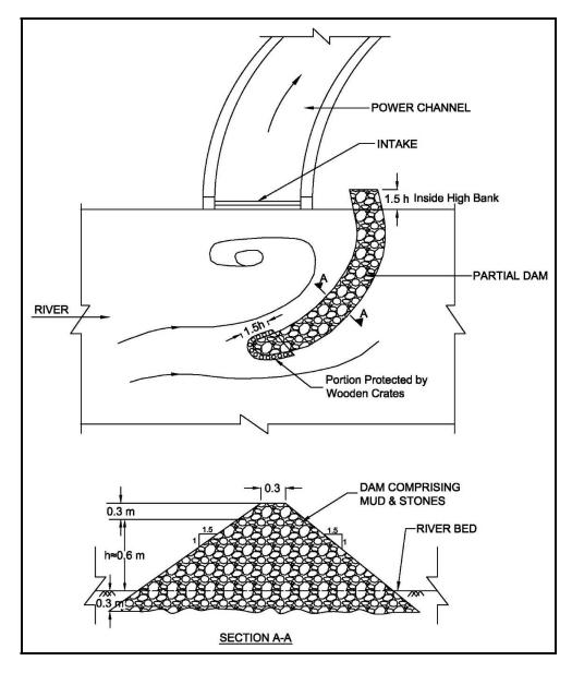
Fig. 2: General Arrangement of Partial Weir
