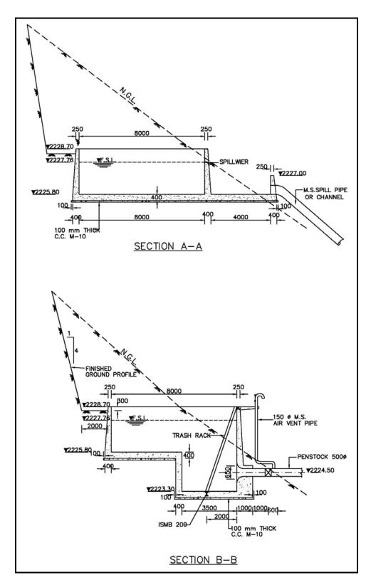
Fig. 57 (b): Typical Details of Forebay (Section)
