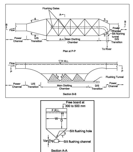
Fig. 54: Schematic Arrangement of Desilting Chamber
