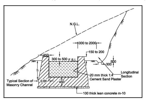
Fig. 44: Typical Section of Masonary Channel
