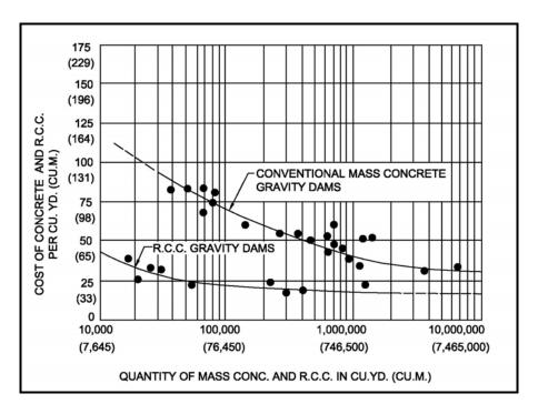
Fig. 10: Comparison of RCC and Mass Concrete Costs (1986 Dollars) (R-37)
