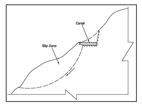
Fig. 37: Typical slip failure due to SHP construction
