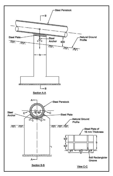
Fig. 60: General Details of CC Saddle Block
