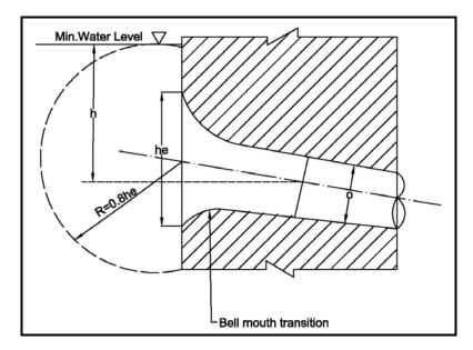
Fig. 36: Sub-mergence Requirement of Pressure Conduits
