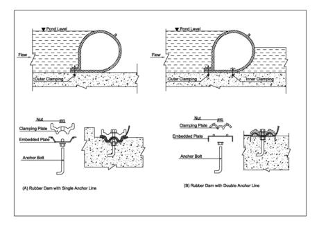
Fig. 14: Typical Cross Section of Inflatable Rubber Dam
