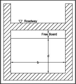
Fig. 52: Typical flume section
