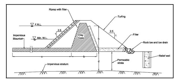
Fig. 27: Section of Earth Dam with Impervious Blanket
