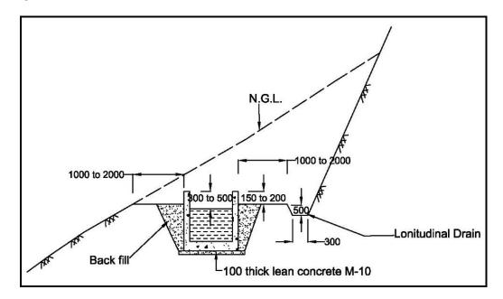
Fig. 42: Typical Section of Open RCC Channel
