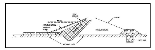
Fig: 25: Typical Earth Dam Section with Foundation Pervious to Large Depth
