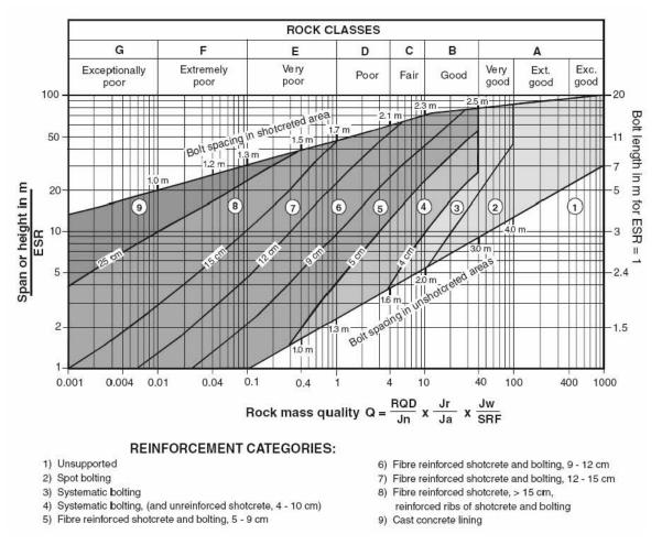
Fig. A1: Estimated Support Categories Based on the Tunneling Quality Index Q (Source: The Development of Rock Engineering by Evert Hoek)
