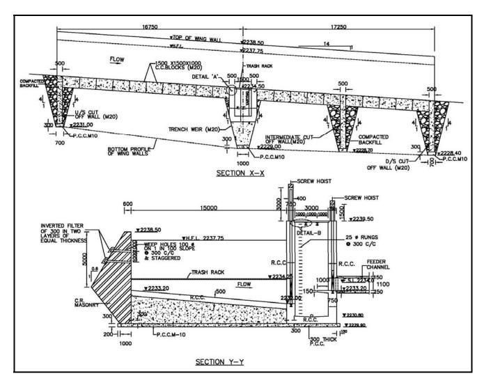
Fig. 5 (b): Typical Details of Trench Weir (Sections)
