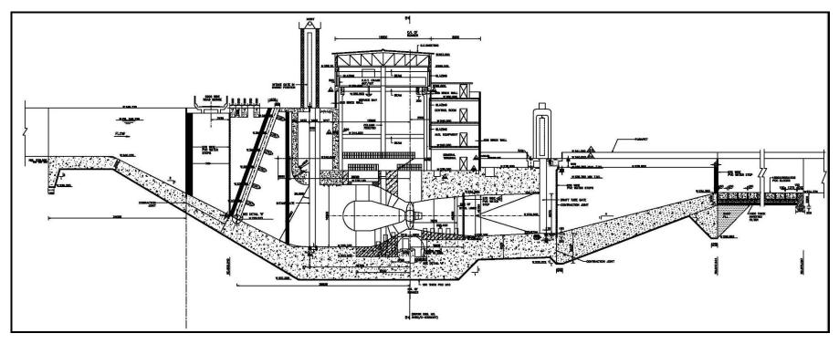
Fig. 66: Typical Transverse Section of Power House with Bulb Turbine
