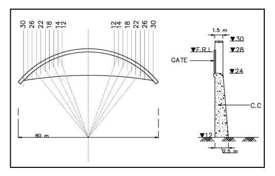
Fig. 13: Typical Plan and Section of Arch Dam
