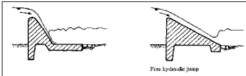
Fig. 2: Dammed hydraulic jump; Free hydraulic jump
