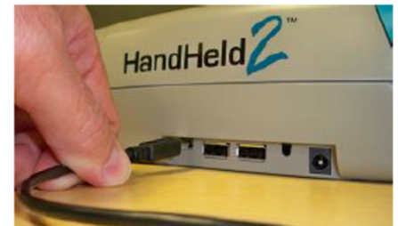
Figure 89: Mini USB plug connects to the instrument
