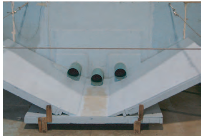
Figure 5-5(G). Three-barrel, 2D horizontal spacing, 0.5D depressed culvert with a trapezoidal channel approach.
