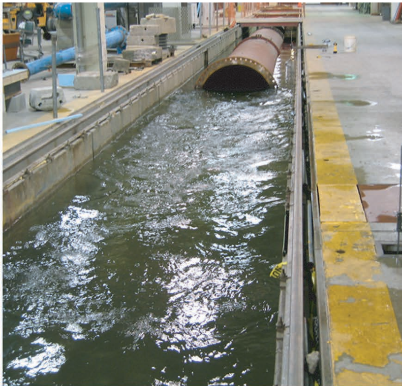
(60-inch diameter pipe exit loss test)
