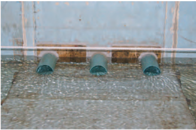
Figure 5-5(C). Three-barrel, 3D spacing with reservoir approach.
