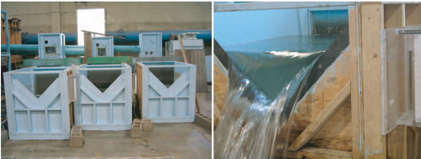
Figure 5-3. V-notch weir/tail box assemblies.
