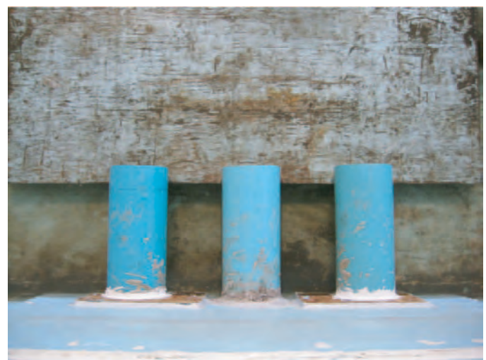
Figure 5-5(B). Three-barrel, 2D spacing with reservoir approach.
