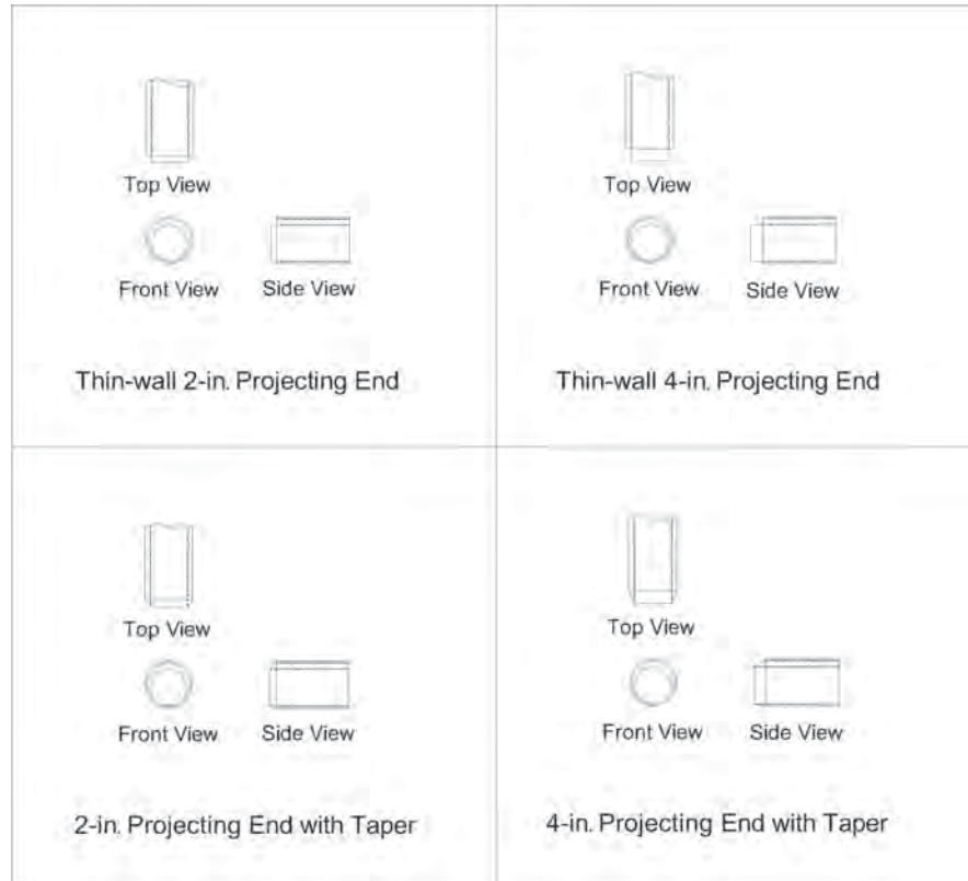
Figure 3-2. Slip-lined culvert inlet end treatments.
