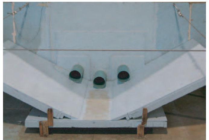
Figure 5-5(H). Three-barrel, 3D horizontal spacing, 0.5D depressed culvert with a trapezoidal channel approach.
