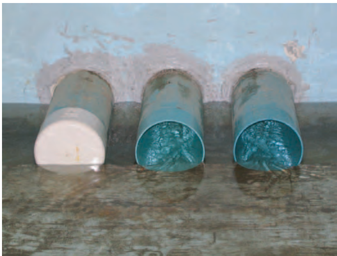
Figure 5-5(A). Two-barrel, 1.5D spacing with reservoir approach.
