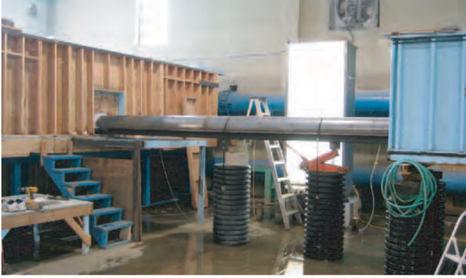
Figure 2-8. Culvert test setup.
