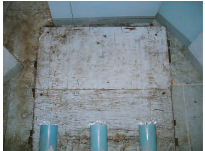
Figure 5-5(F). Three-barrel, 3D spacing with a non-uniform approach flow.
