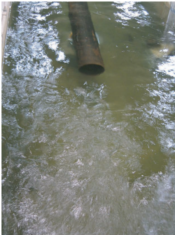
(12-inch diameter pipe exit loss test)
