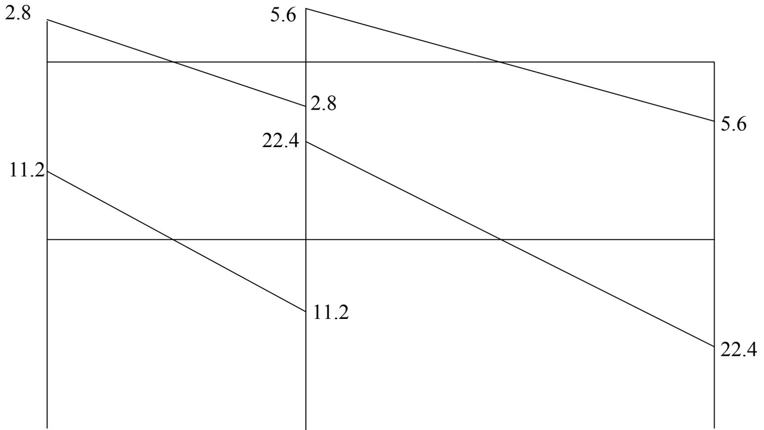
Fig. 1.13. Bending Moment Diagram For Beams.
