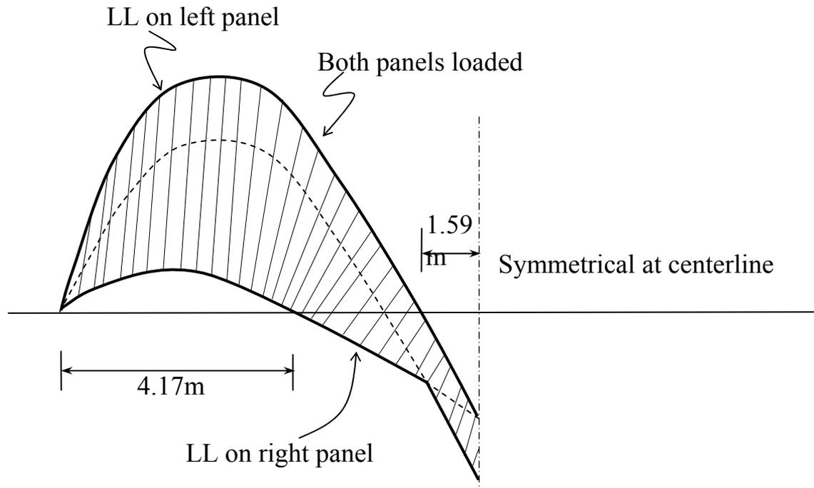
Fig. 10.64. Shear and Moment Envelopes for Beam of Example 10.16.
