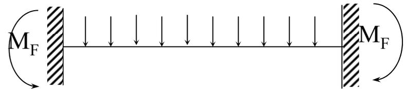
Fig. 1.6. Fixed End Moment For a Beam Segment Having UDL.
