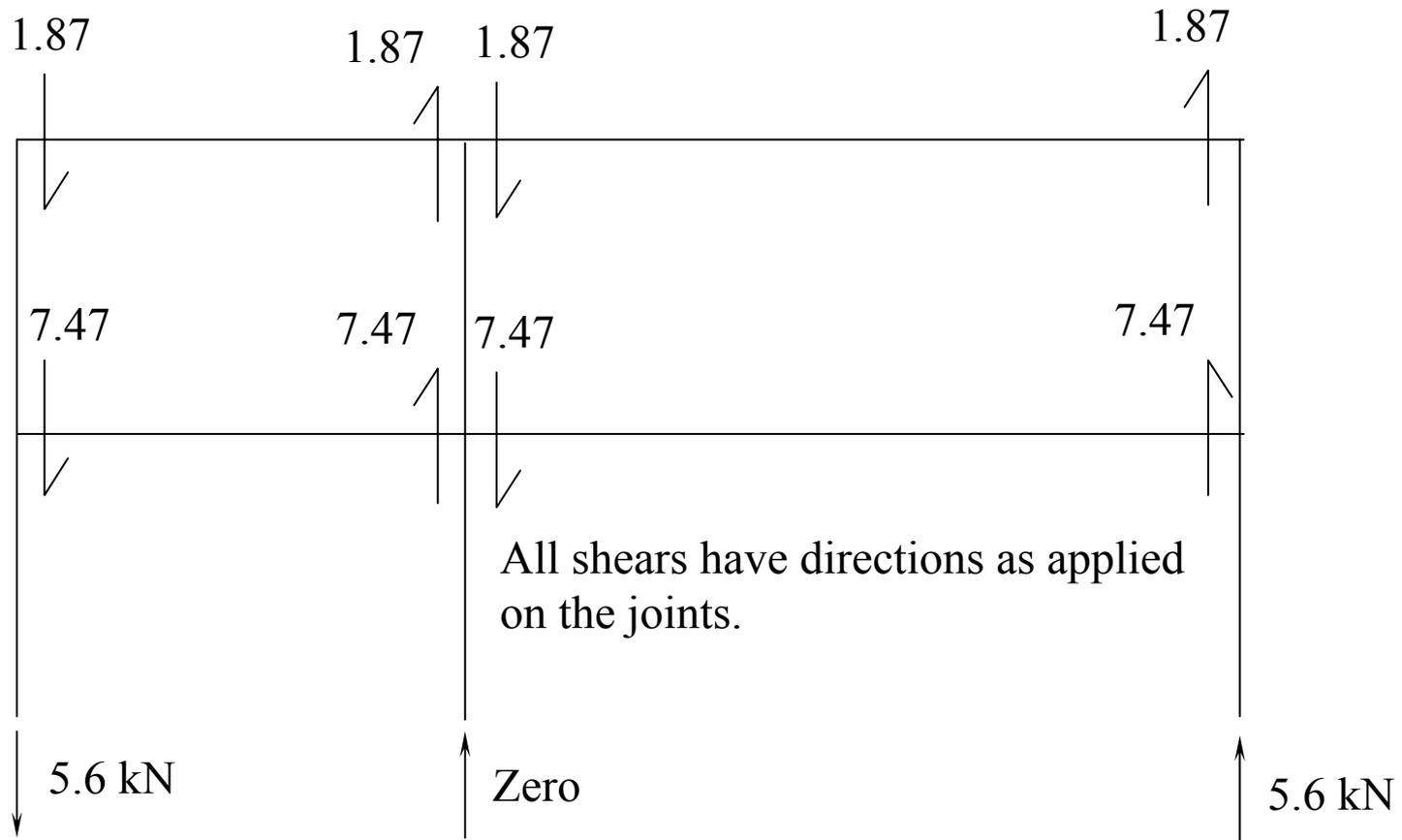
Fig. 1.14. Shear Force Diagram For Columns.
