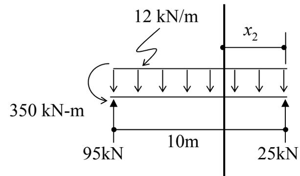
Fig. 10.62. Solution of Example 10.16 For Case-II.
