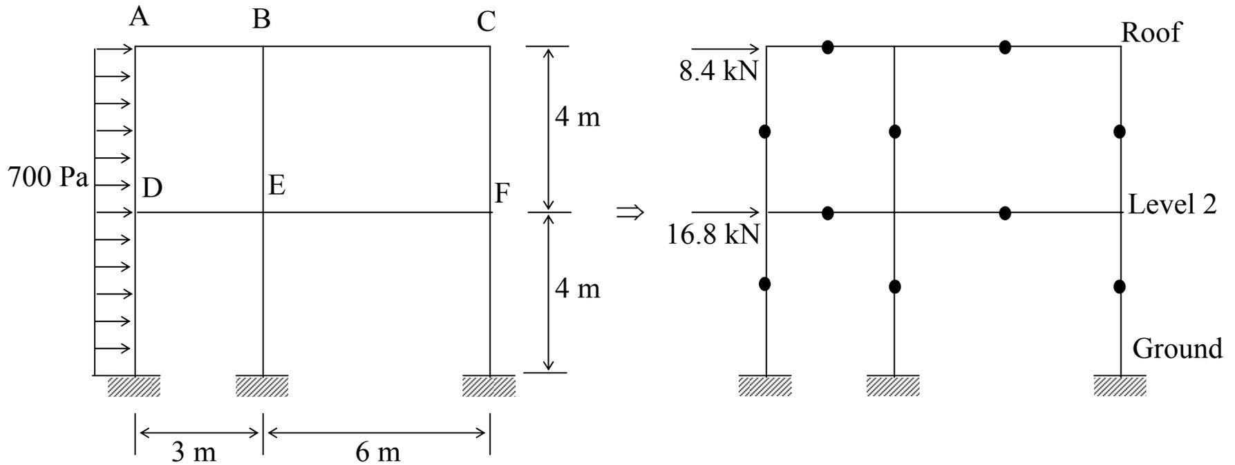
Fig. 1.8. Data And Position Of Inflection Points For Example 1.2.
