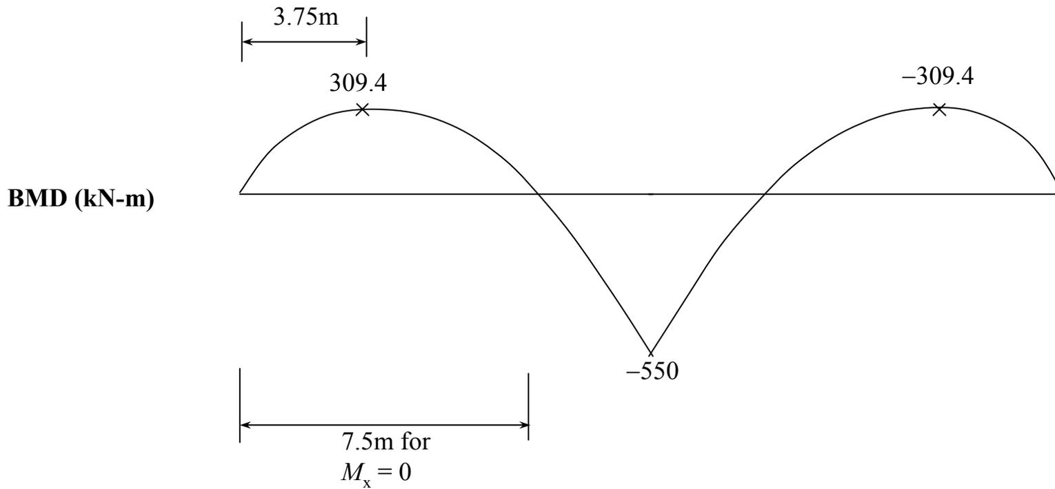
Fig. 10.61. SF and BM Diagrams for Case-I of Example 10.16.
