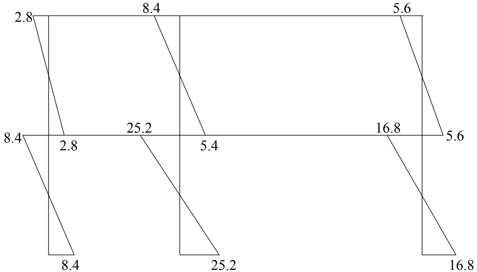
Fig. 1.12. Bending Moment Diagram For Columns.
