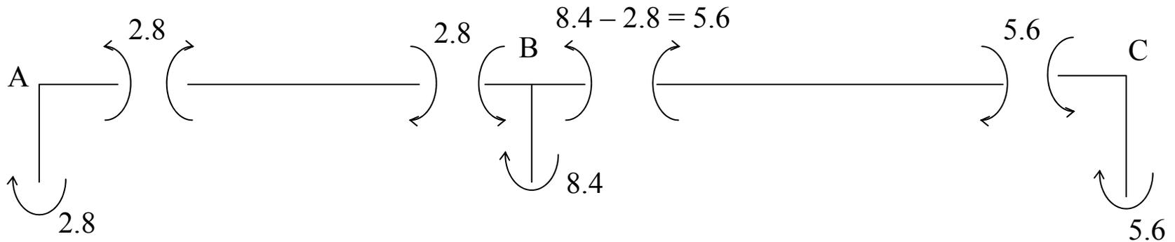
Fig. 1.10. Calculation of Beam Moments For Upper Floor.
