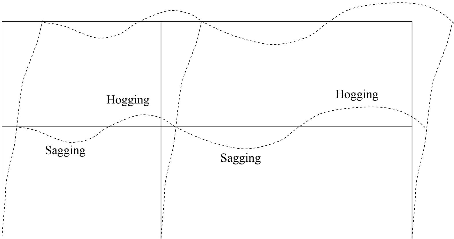
Fig. 1.15. Approximate Elastic Curve Diagram For The Frame Due to Wind Load Showing Sense of Bending.
