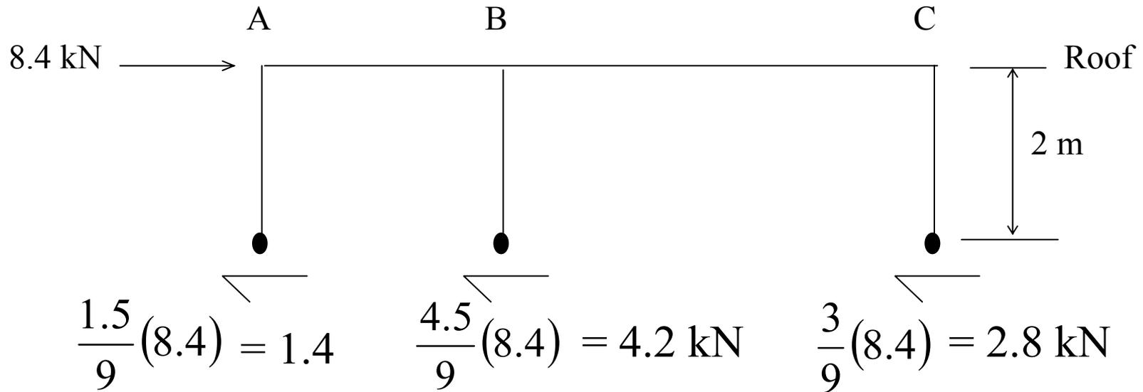
Fig. 1.9. Columns Shears For Upper Floor.
