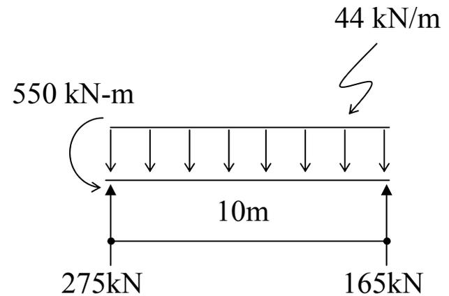
Fig. 10.60. Free Body Diagrams For Beam of Example 10.16.
