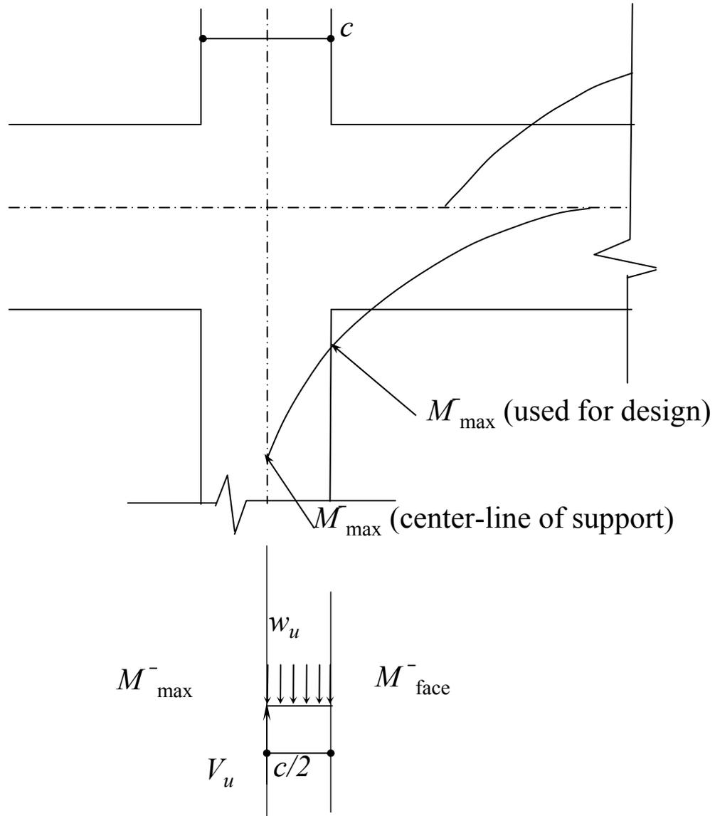
Fig. 10.57. Moment Envelope Near Beam Joint With Column.
