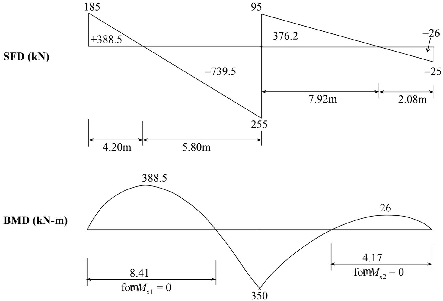
Fig. 10.63. SF and BM Diagrams for Case-II of Example 10.16.
