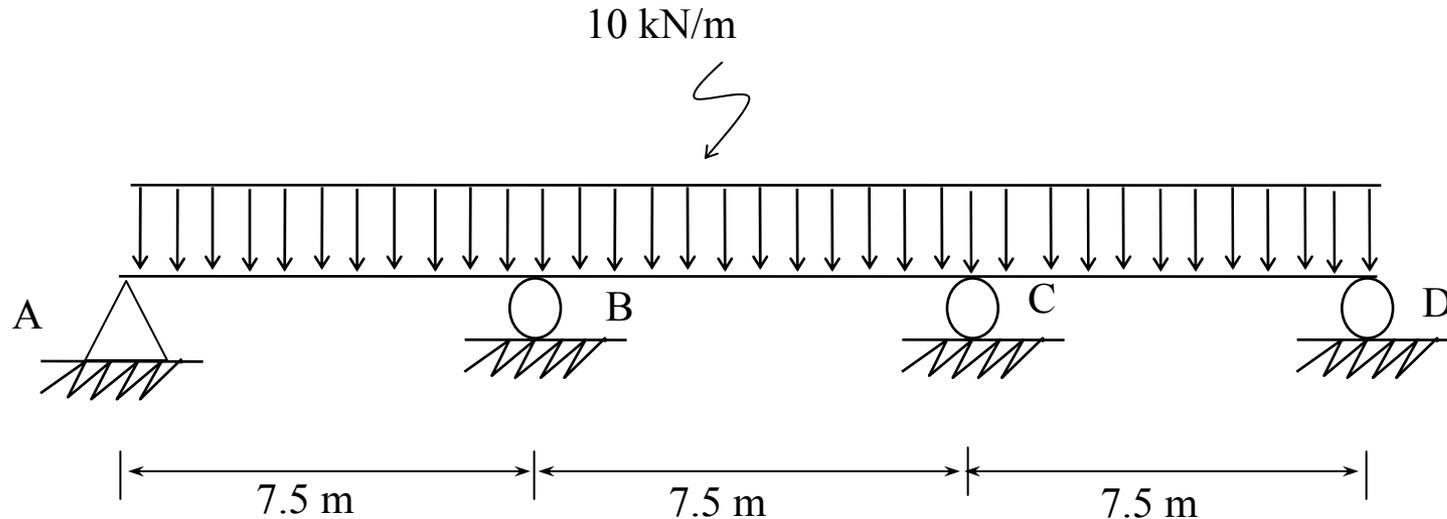
Fig. 1.5. Continuous Beam For Approximate Analysis.
