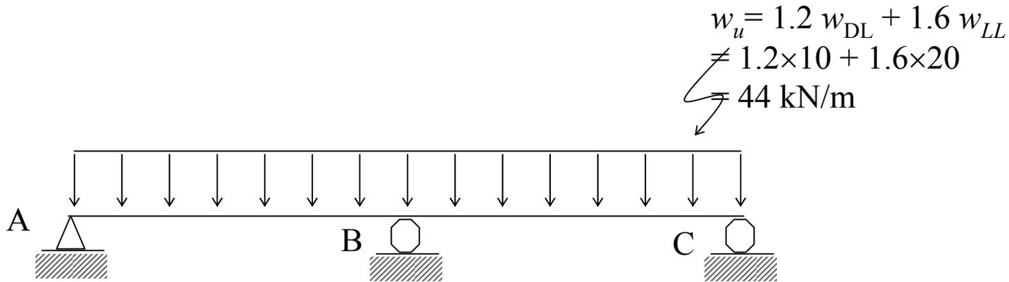
Fig. 10.59. Loading of Case-1 for Beam of Example 10.16.
