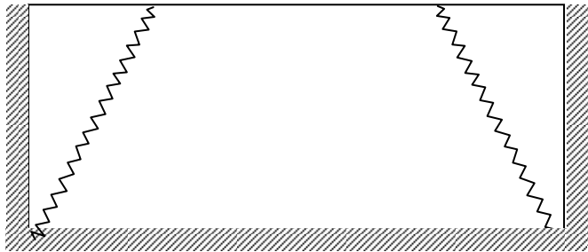
m) Rectangular Slab Simply Supported On Three Sides Having Large Aspect Ratio
