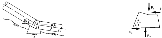
Fig. 5.27 – Resultant forces produced by weight, pressure and change in momentum.
