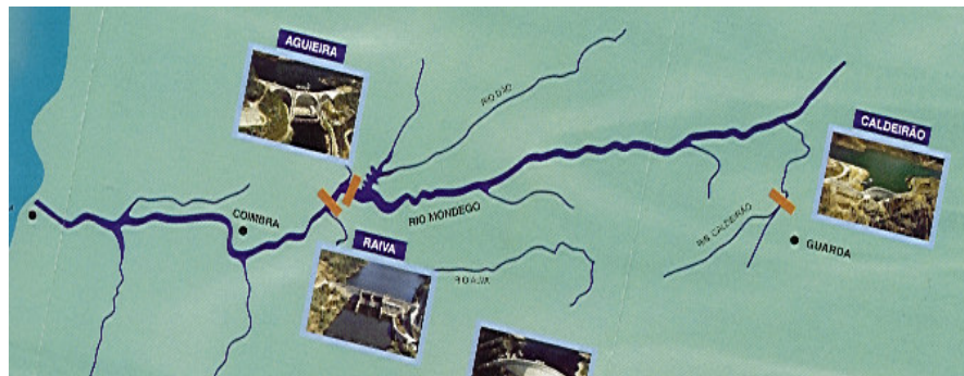
Fig. 2.4 – Example of a cascade scheme of large dams (courtesy of EDP).
