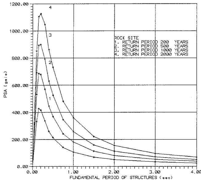
**Fig. 6.16: Design spectra (PSA), rock site, Jinnah HPP**
