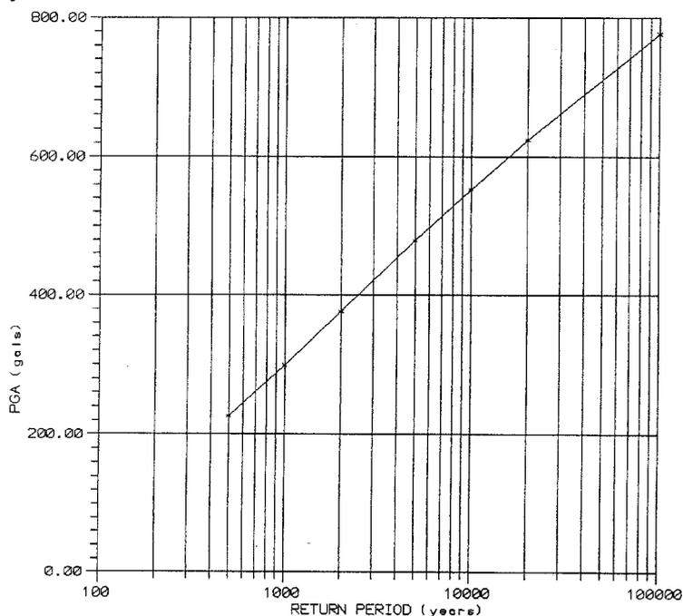
Fig. 6.12: Peak ground acceleration, Jinnah HPP
