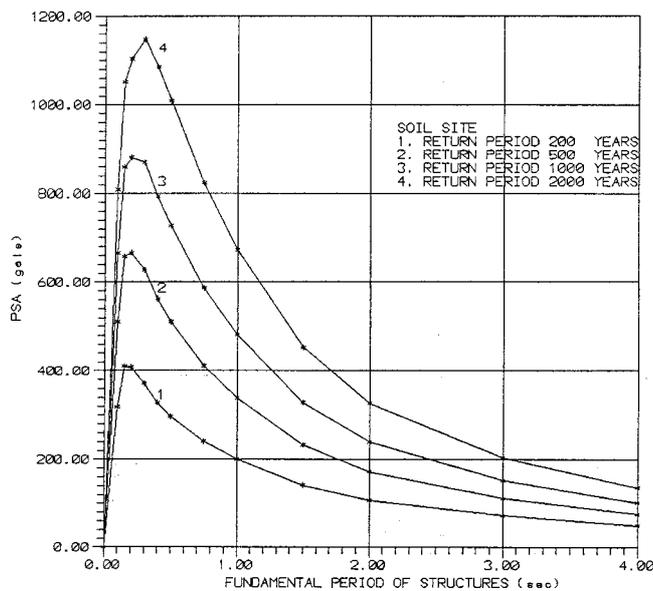
**Fig. 6.15: Design spectra (PSA), soil site, Jinnah HPP**
