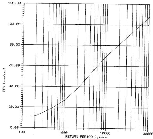
**Fig. 6.14: Peak ground velocity, rock site, Jinnah HPP**
