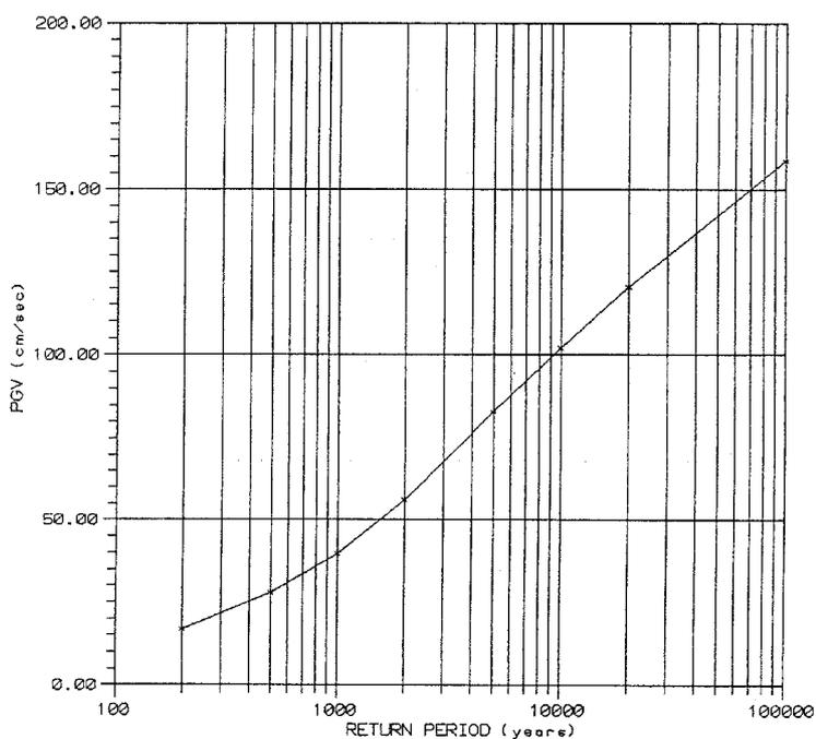
**Fig. 6.13: Peak ground velocity, soil site, Jinnah HPP**
