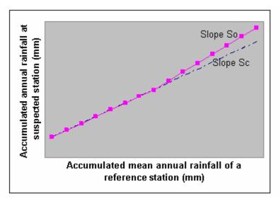
FIGURE 7. A typical example of inconsistent rainfall record
