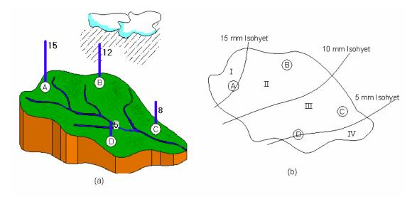
FIGURE 4. Rainfall measurement by the Isohyetal method. (a) Recorded rainfall; (b) Isohyets and the areas enclosed bewteen two consecutive isohyets.
