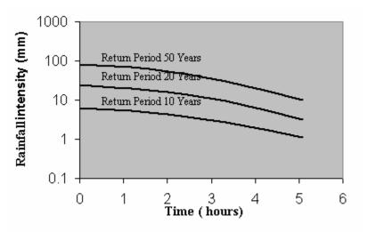
FIGURE 6. A typical rainfall intensity-duration-frequency (IDF) curve
