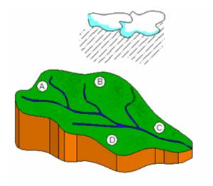
FIGURE 1. A hypothetical catchment showing four raing gauge stations
