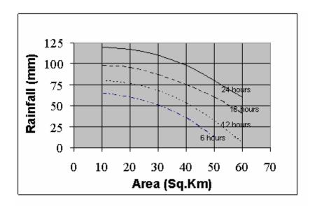
FIGURE 5. A typical Depth-Area-Duration (DAD) curve
