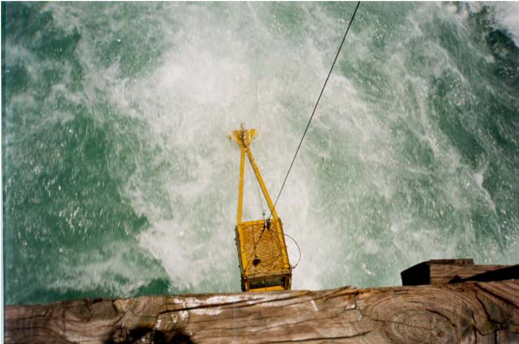
Fig. 4.4: Bed load sampling at mountain river with basket sampler
