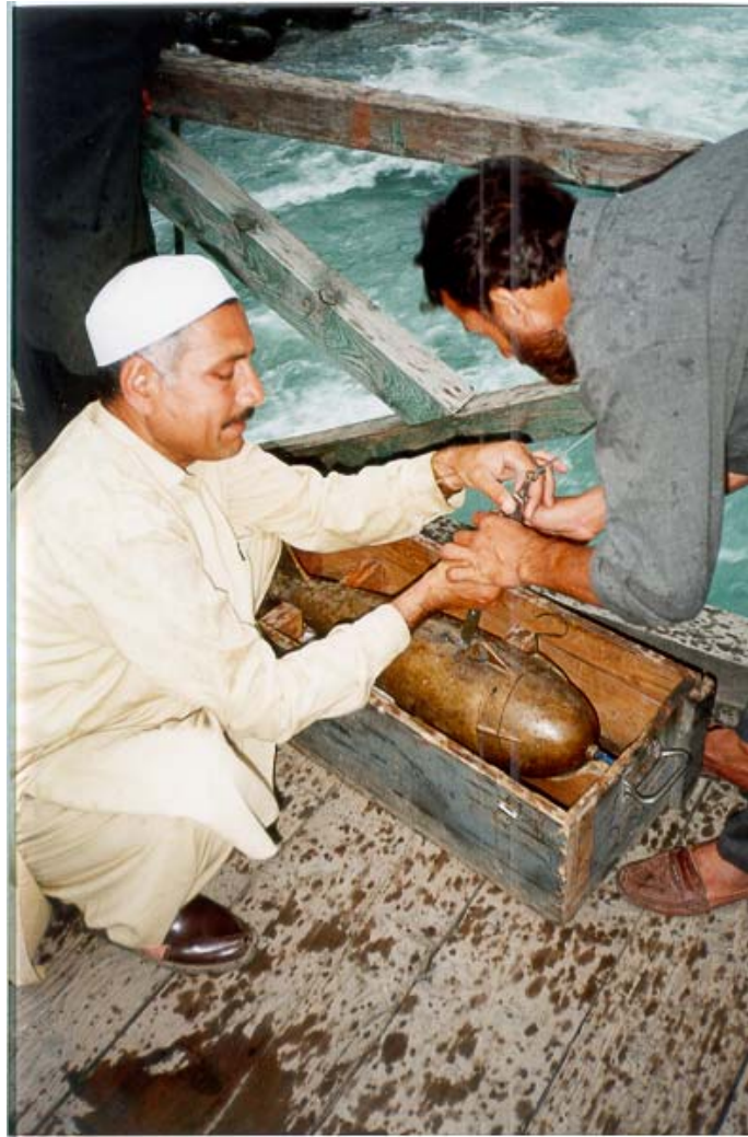
Fig. 4.6: Examples of integrating sampler P-49 during field measurement
