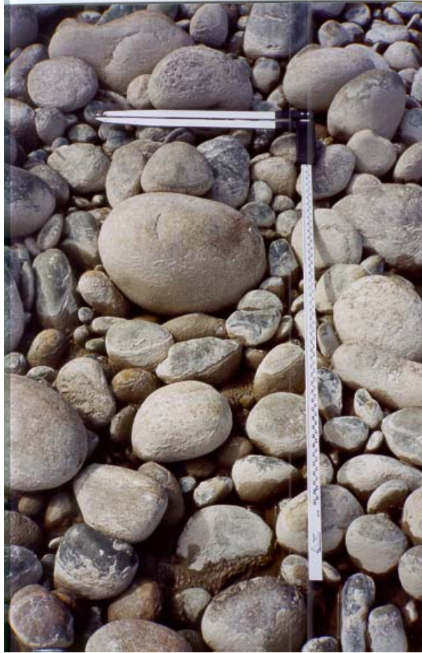
Fig. 4.8: LBN measurement of armour layer
