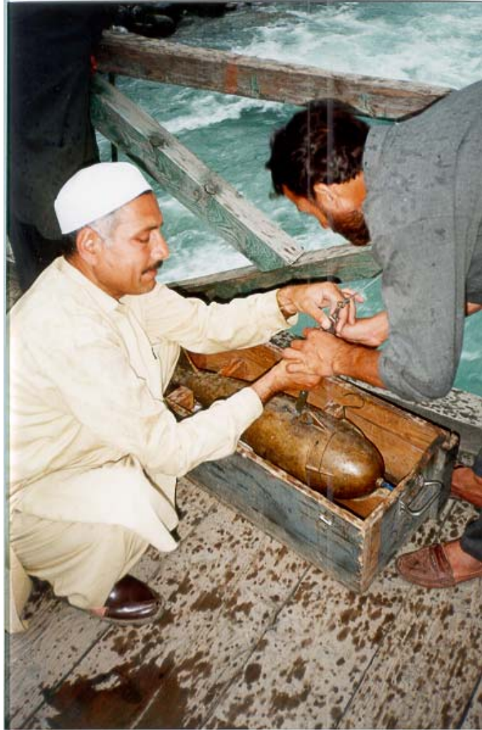
Fig. 4.6: Examples of integrating sampler D-49 during field
