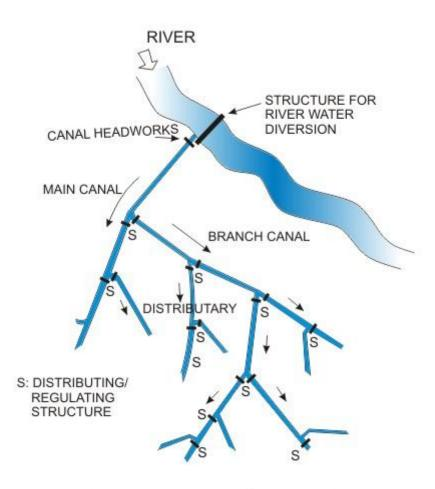
FIGURE 1 : Typical layout of an irrigation canal system
