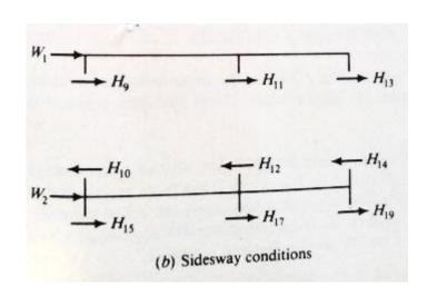
Shear Condition-(Upper Storey)  $H_9+H_{11}+H_{13}+W_1=0$  Shear Condition for Lower Storey  $H_{15}+H_{17}+H_{19}-H_{10}-H_{12}-H_{14}+W_2=0$
