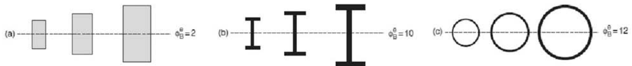
Figure 2.5.1 Schematic pictures of a set of (a) rectangular sections with \phi_B^e = 2 ; (b) I-sections with \phi_B^e = 10 ; and (c) tubes section with \phi_B^e = 12 .
