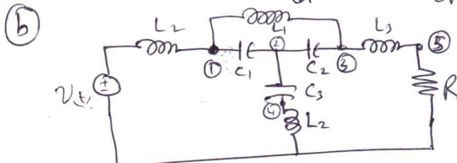
Node-1  $\frac{1}{L_2} \int (V_1 - V_{bt.}) dt + \frac{1}{L_1} \int (V_1 - V_3) dt + C_1 \frac{d(V_1 - V_2)}{dt} = 0$
