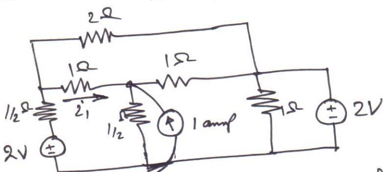
Apply Node Analysis, convert Voltage source 2V, in series with  $1/2 \Omega$  into equivalent Current source
