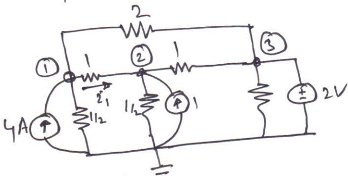
No - Need to write equation for Node-3, as  $V_3 = 2$  Volt.
