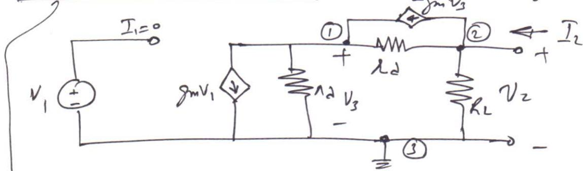
$$g_m V_1 + \frac{V_1}{R_d} + \frac{V_1 - V_2}{R_d} - (-g_m V_3) = 0$$
