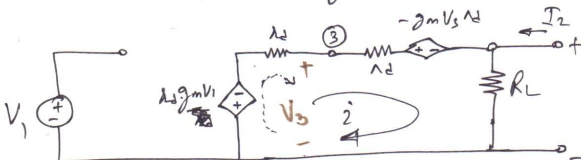
$$\lambda_d g_m V_1 + (-g_m V_3 \lambda_d) + i \lambda_d + i \lambda_d + R_L i = 0$$
