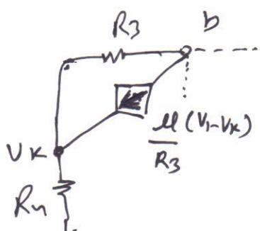
$$\frac{V_b - V_K}{R_3} + \frac{V_b - V_d}{R_5} + \frac{V_b - V_c}{R} = 0$$
