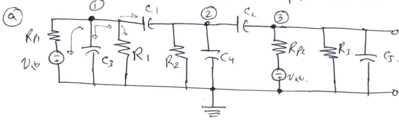
Node-1  $\frac{V_1 + V_{bt.}}{R_{P1}} + C_3 \frac{dV_1}{dt} + \frac{V_1}{R_1} + C_1 \frac{d(V_1 - V_2)}{dt} = 0$
