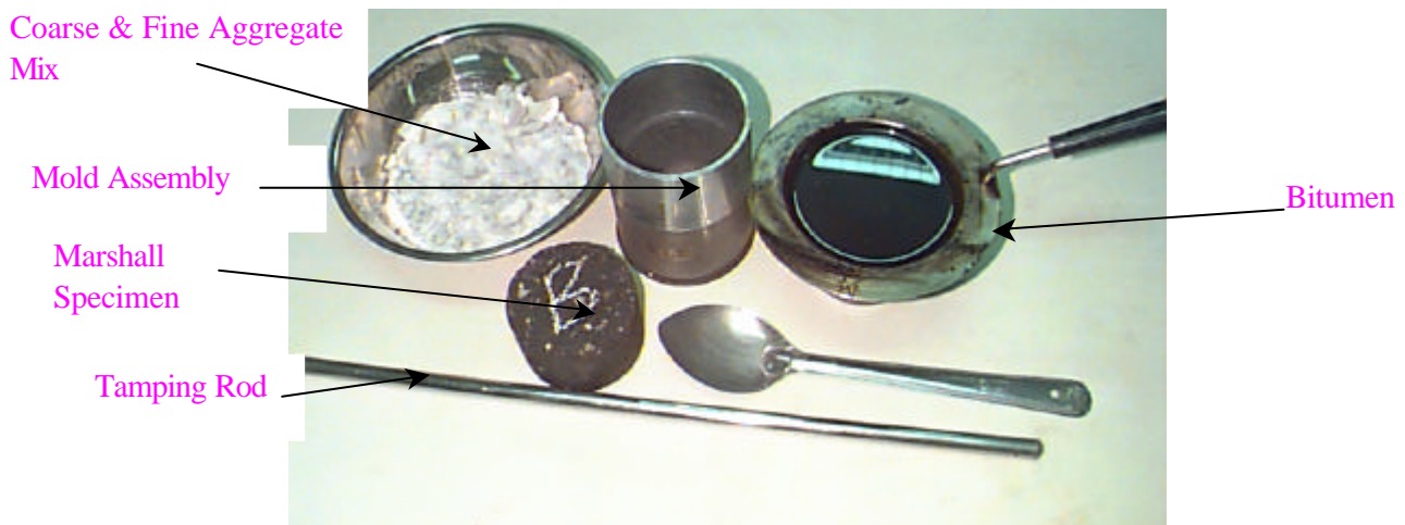
Figure 11.3 Test Specimen Preparation
