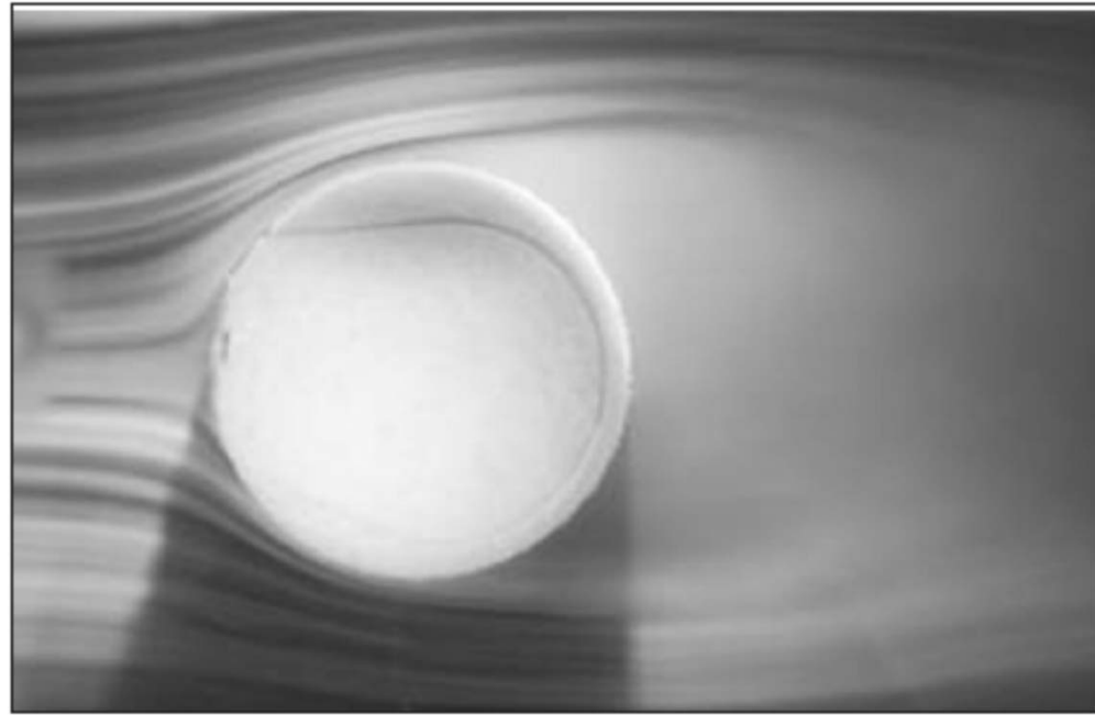
External flow over a tennis ball, and the turbulent wake region behind.
