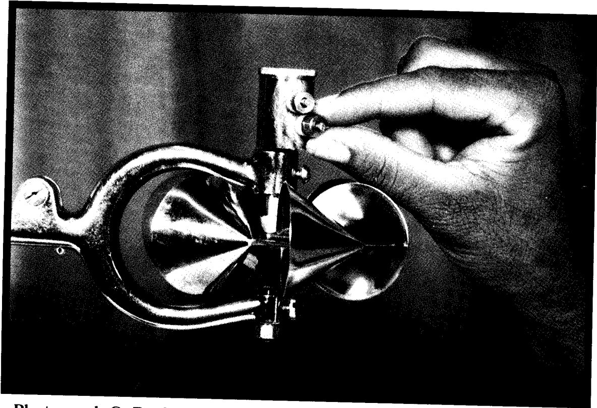
Photograph C. For high velocity measurement use lower nut connection.
