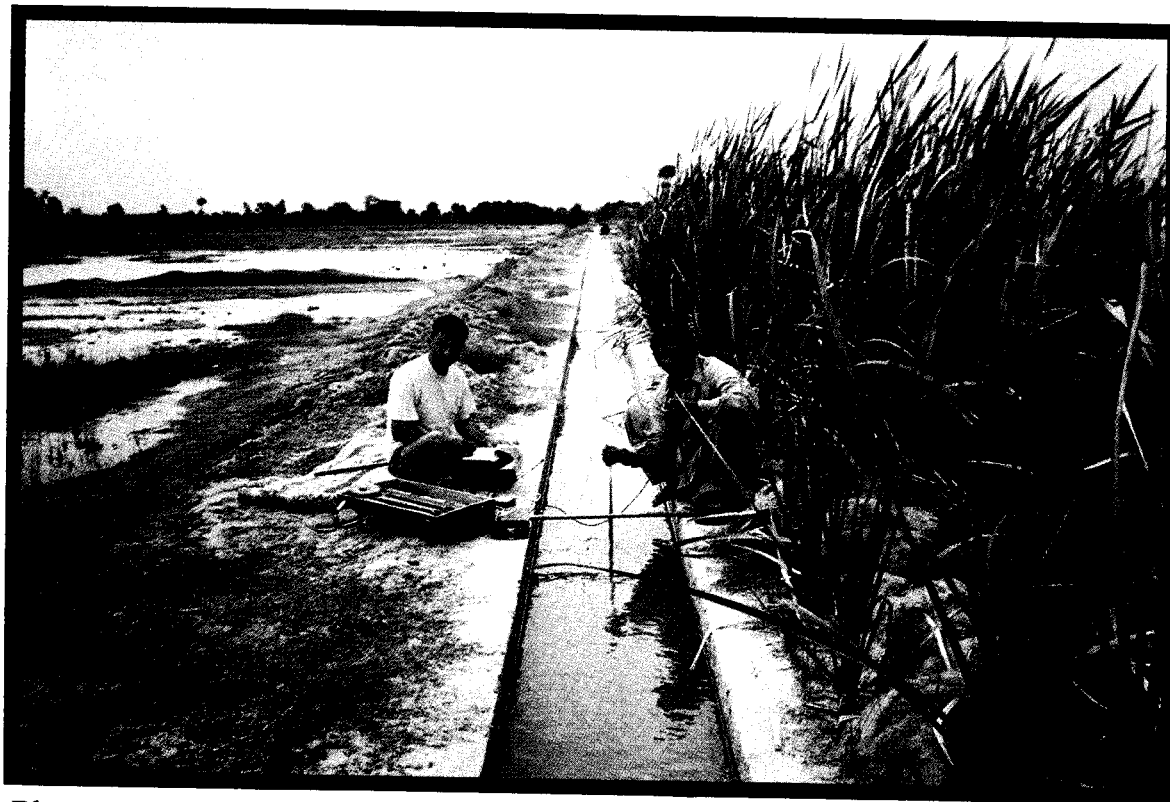
Photograph B. Using a Pygmy current meter in a lined rectangular cross-section of a watercourse.
