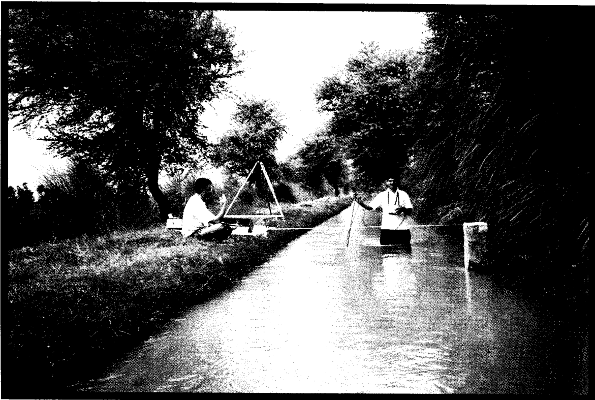
Photograph M. The Notekeeper signaling the Hydrographer regarding the verticalness of the wading rod.
