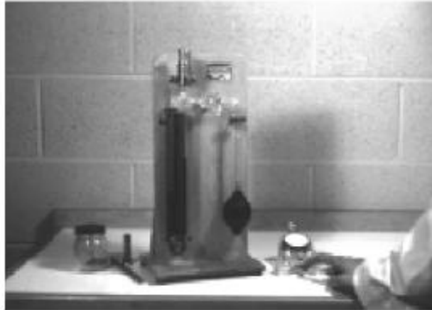
Blaine, ASTM C 204 ( \text{m}^2/\text{kg} )
