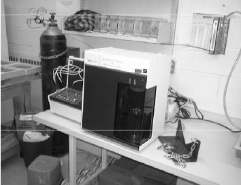
Nitrogen adsorption Surface area
