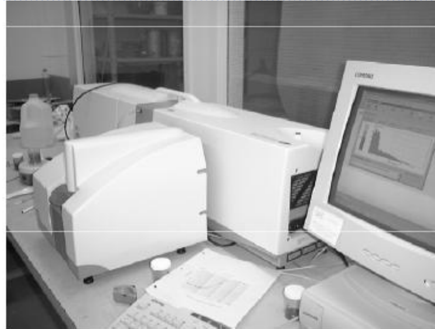
Laser diffraction particle size analysis
