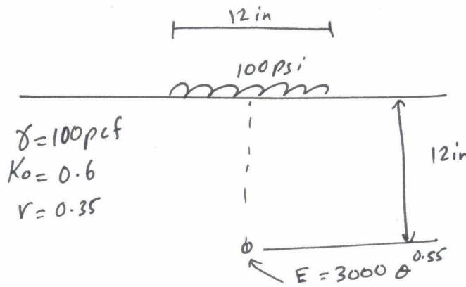
Determine max. surface displacement.
