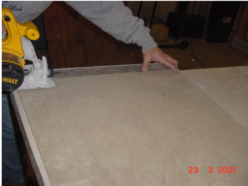
Fig.38. Cutting the acrylic to make the gate face
