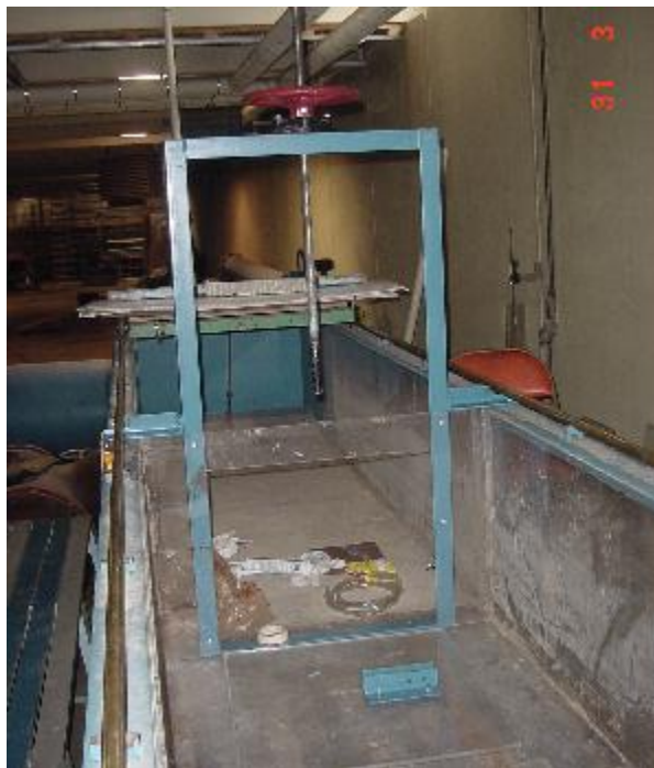
Fig.40. Gate after installation in the rectangular flume
