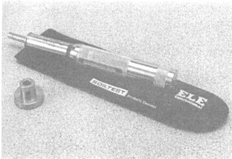
Figure 8.35 Pocket penetrometer (PP), a hand-held device which indicates unconfined compressive strength (Courtesy: Soiltest, USA)
