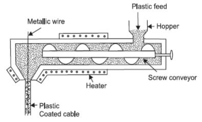
material is forced out of a notch having the shape of the finished product needed. Thermoplastic rods and tubes are extruded through dyes. If, however, something is to be provided with the plastic covering like insulation of electric wires and cables then the same is drawn through a dye.
