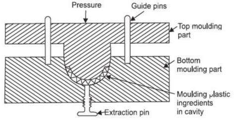
In this process the raw material is placed in the mould cavity and both parts of the mould are subjected to high pressure along with the simultaneous heating of the mould.
