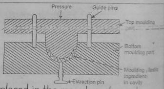
In this process the raw material is placed in the mould cavity and both parts of the mould are subjected to high pressure along with the simultaneous heating of the mould.
