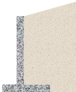
Cantilever retaining wall
