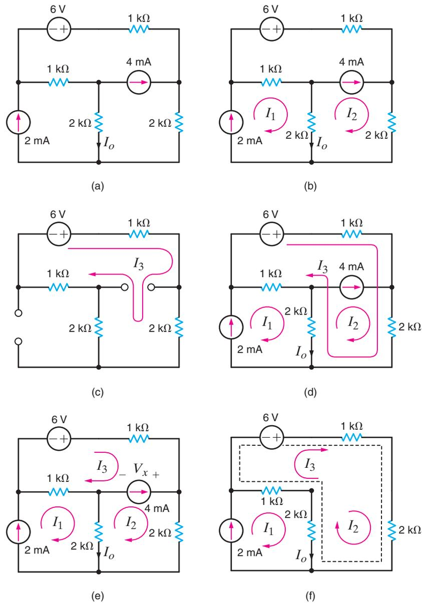
Figure 3.24 Circuits used in Example 3.16.
