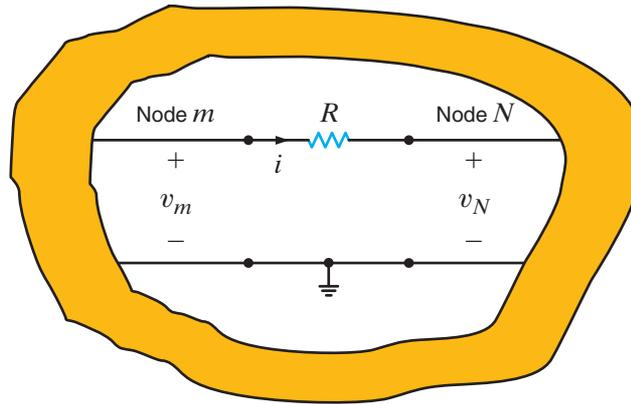
Thus, as a general rule, if we know the node voltages in a circuit, we can calculate the current through any resistive element using Ohm's law; that is,
