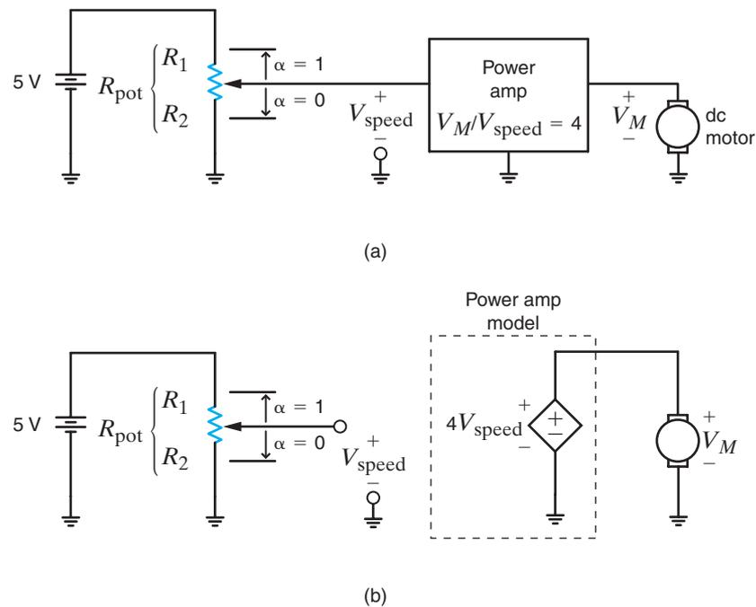
Figure 3.30 (a) A simple dc motor driver and (b) the circuit model used to analyze it.
