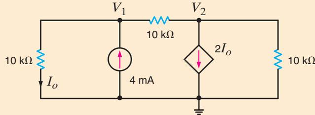
**E3.4** Find the voltage  $V_o$  in the network in Fig. E3.4.
