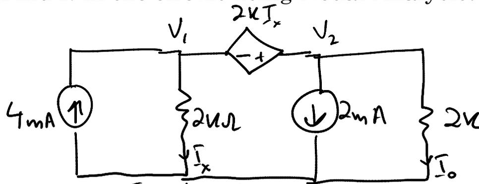
Using KCL at nodes 2 and Forming a controlling equation
