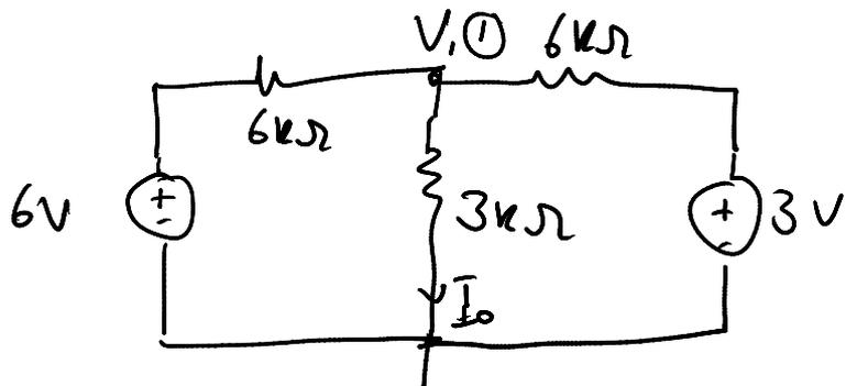
$$\frac{V_1 - 6}{6k} + \frac{V_1}{3k} + \frac{V_1 - 3}{6k} = 0$$
