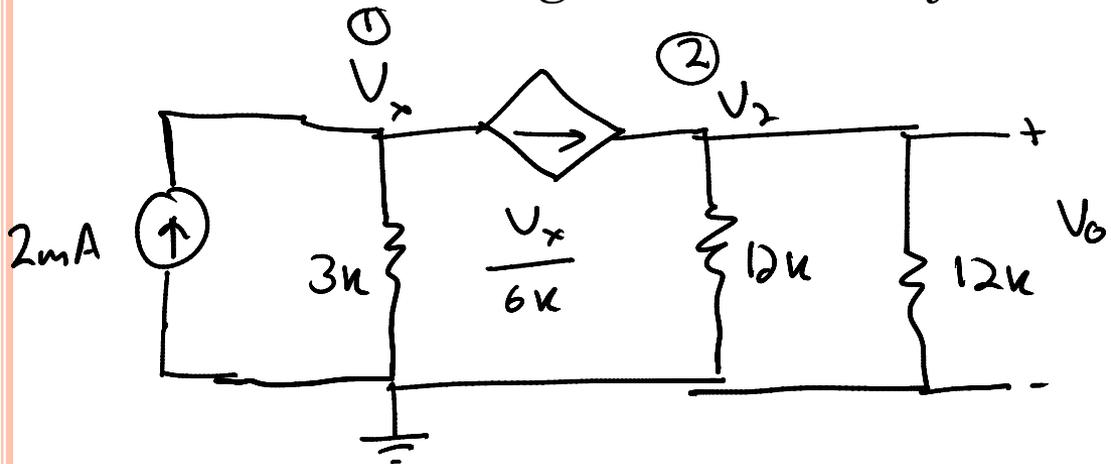
For this Circuit, We need to Overlook the node with dependent Source and form equations round it. We use KCL at Nodes 1 and 2 and derive the equations based on Current flow.
