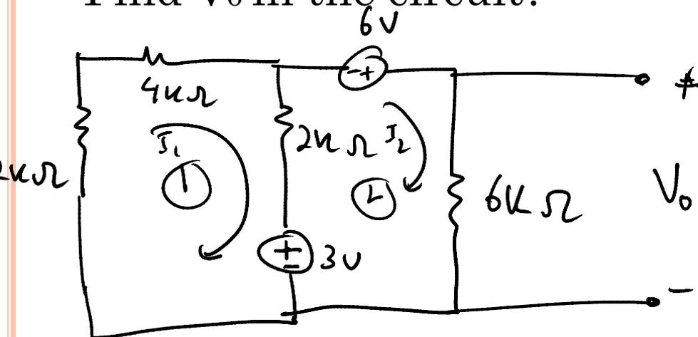
Using KVL at loops 1 and 2, we form KVL equations using the current and Components in the loops in terms of The loop currents.
