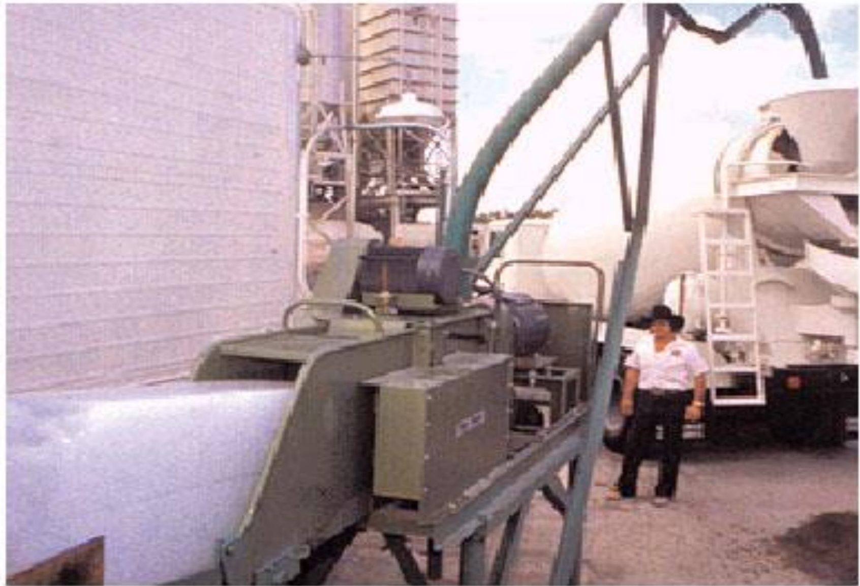
Fig. 13-6. Substituting ice for part of the mixing water will substantially lower concrete temperature. A crusher delivers finely crushed ice to a truck mixer reliably and quickly. (44236)
