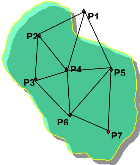
**Step 2:** Join location of the raingauges to form a network of triangles
