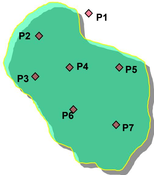
**Step 1:** Draw the area concerned to a suitable scale, showing its *boundary, locations of the raingauges in the area and outside but close to the boundary*
