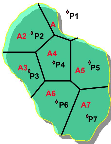
**Step 4:** Delineate the formed polygons and measure their areas using a planimeter or by converting them into smaller regular geometric shapes (i.e. triangles, squares, rectangles, etc.)
