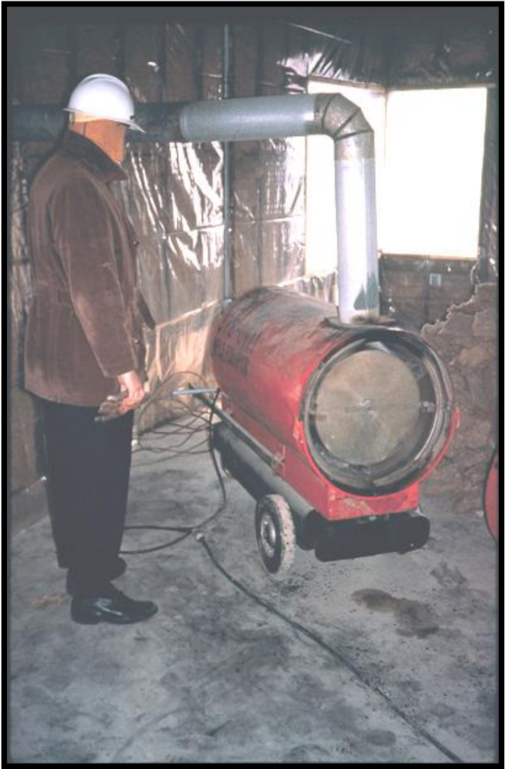
An indirect-fired heater. Notice vent pipe that carries combustion gases outside the enclosure.
