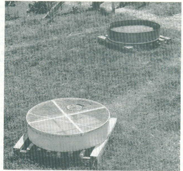
FIGURE 4.3.1 U.S. Weather Bureau Class A evaporation pans with screen in the foreground, and without screen in the background.
