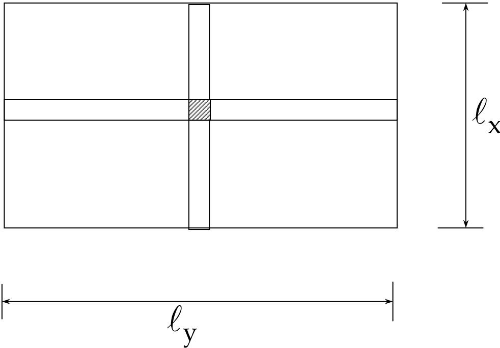
Design Strips in a Two-Way Slab.
