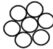
Fig. 19.3. A Seven Wire Strand.
