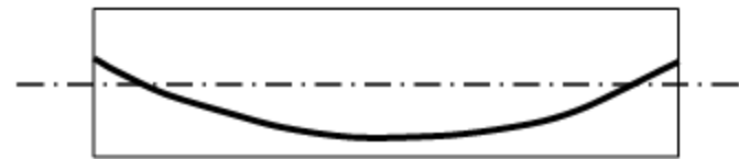
(b) Parabolic Tendon
