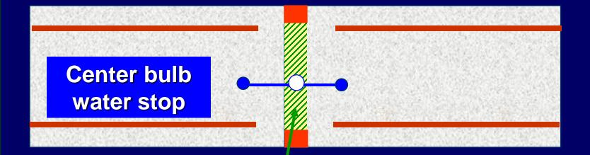
Non absorbent joint filler in an initial gap for expansion
