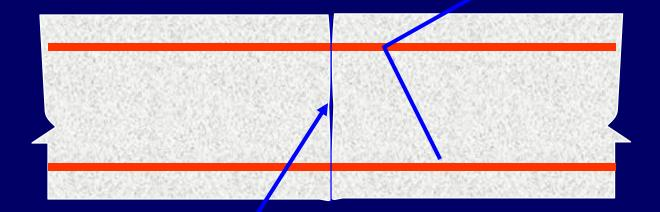
Concrete joint surface prepared for subsequent continuity
