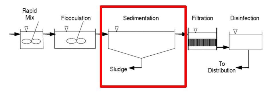
It is a process of **separation of unstable** and **destabilized suspended particles** from suspension by the **force of gravity**.
