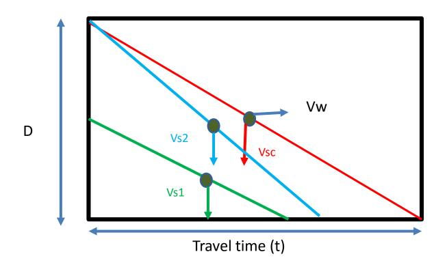
Particles having settling velocity (Vs) greater than Critical velocity (Vsc) will be removed 100% regardless of the position of particle at inlet
