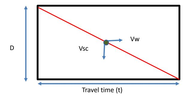
Particle will settle down by travelling a vertical distance (D) in a time (t) with a settling velocity (Vsc):
