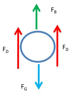
After an initial transient period, the acceleration dV<sub>s</sub>/dt becomes zero and the settling velocity becomes constant
