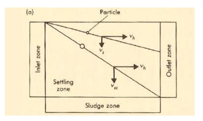
All particles with  $V_s > V_c \rightarrow will$  be completely settled. Particle with  $V_s < V_c \rightarrow will$  be removed in the ratio  $V_p / V_c$  • Surface over flow rate(SOR) is a critical design
