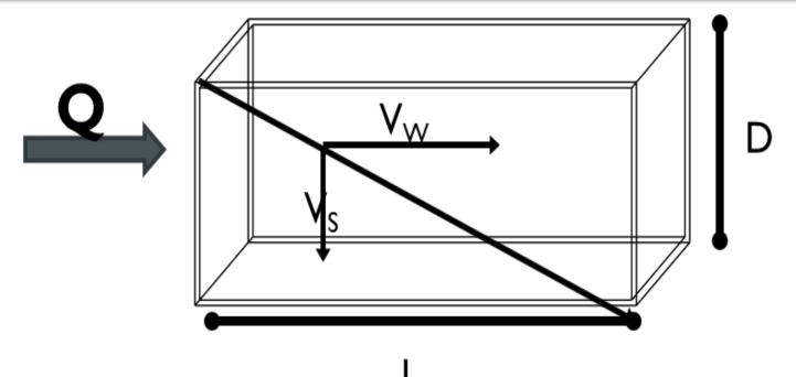
L=length of settling zone D=depth of settling zone W=width of settling zone Vs=settling velocity of particle Vw=horizontal velocity of water Q=inflow to tank V=volume of tank As=surface are of tank
