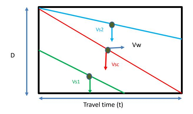
Particles having settling velocity (Vs)less than Critical velocity (Vsc) will be removed in the ratio of Vs/Vsc.May also depend on their position at inlet.
