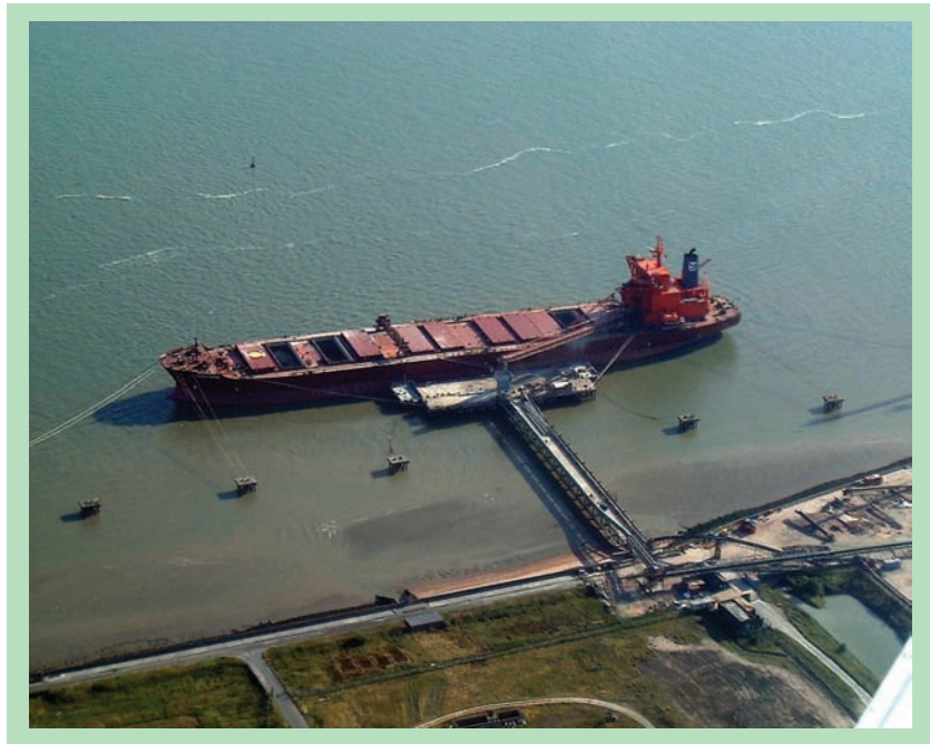
Figure 4.50 Aggregate wharf and the one of the Foster Yeoman self discharging vessels. Photograph by Samantha Cooke.
