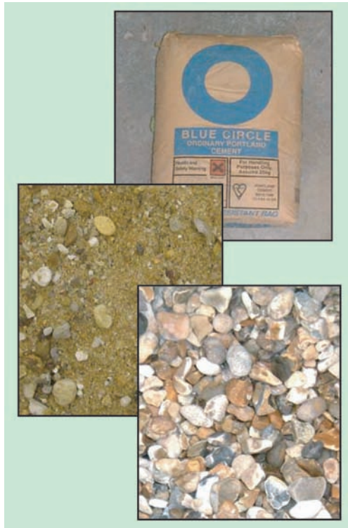
Figure 4.47 Main components of dense concrete.
