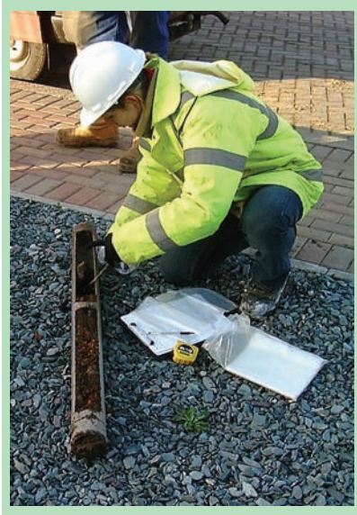
Figure 4.44 Geologist inspecting an undisturbed soil sample.
